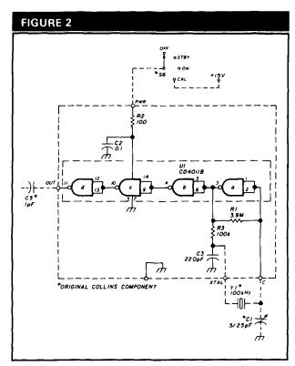
100-kHz crystal calibrator schematic.
