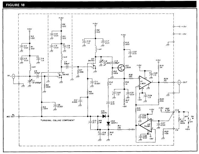
Noise limiter i-f and noise pulse detector schematic.
