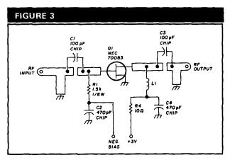
Schematic diagram of GaAsFET amplifier.
