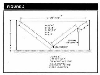
Inverted Delta Loop for 80 meters. This antenna provides a good low angle of radiation and is excellent for Dxing.
