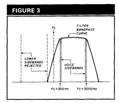
A crystal filter can be used to pass one sideband and reject the other. The suppressed RF carrier ( $F_c$ ) is usually placed on one slope of the filter's response curve as shown in order to pass the band of frequencies in the sideband.
