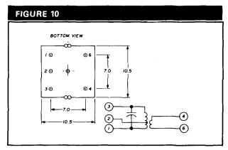
Mounting dimensions for the Toko transformers. The measurements are in mm. Drill the center hole for a standard-sized screw to hold the template on your circuit board while drilling.
