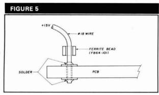
Ferrite bead placement on the +15 volt Vdc line.
