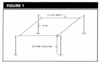
Full-wave horizontal loop with dimensions. This antenna is an excellent high-angle radiator and should be very useful for local communications.
