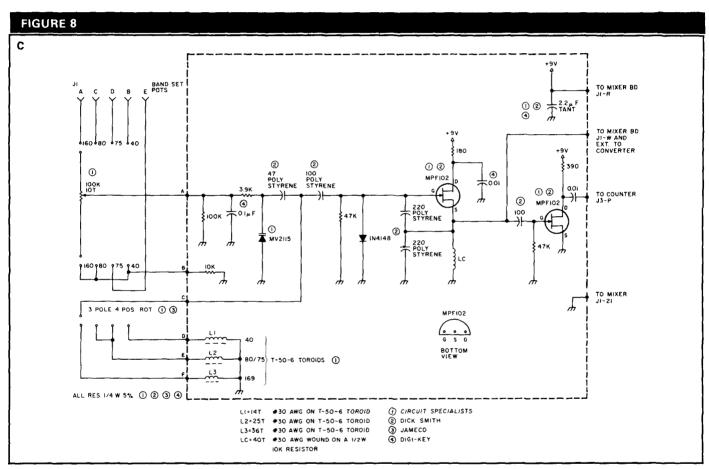
Oscillator board schematic.
