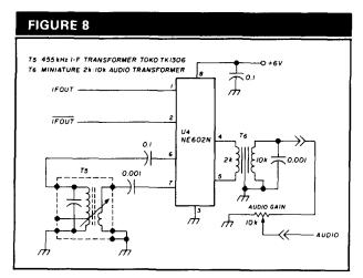
5×8 product detector/second oscillator. See text for comments on the capacitor at U4-7. The oscillator could be made tunable by adding a varicap diode across T5, using the circuit of fig. 4.
