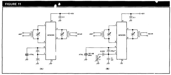
Simple converters using the NE602N. (A) shows the circuit for fundamental crystals; (B) shows the circuit for overtone crystals. Component values for (A) depend on the frequency being converted. The (B) circuit oscillator is appropriate for 10 meters. L1 and C1 should be rough-tuned to 30 MHz, to assure operation on the proper c retone frequency.
