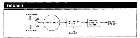
A simplified diagram of a system to select between upper and lower sideband by switching oscillator crystals. The 8.9985 MHz crystal provides upper sideband; the 9.0015 MHz one is for the lower sideband.
