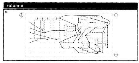
Oscillator board foil-side connections.
