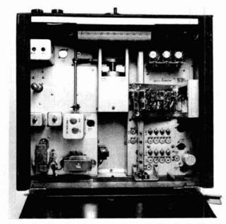
Top inside view showing exposed noise limiter, i-f circuit, and added 3.1-kHz mechanical filter.
