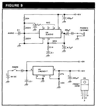
Audio and regulator circuits for both the  $3\times8$  and  $5\times8$ designs.
