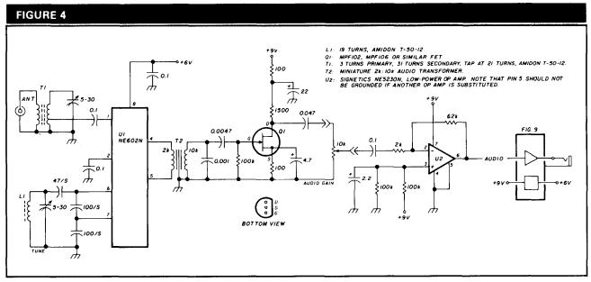
Schematic of the  $3 \times 8$  direct conversion receiver. The tuned circuit values shown are for the 10-meter version, but they are easily scaled for other frequencies. Whole numbered capacitor values are pF, except for polarized capacitors which are  $\mu$ F. Decimal capacitors are also μF. Components marked /s (stable) are polystryene, silver mica, or NPO ceramic. The audio and regulator circuits are "recycled" from fig. 9.
