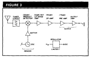
Block diagram of the  $3\times 8$  direct conversion receiver. Having more than one function per chip is advantageous.
