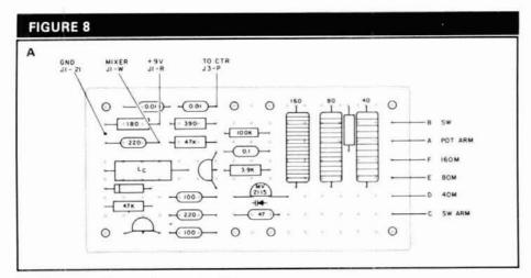
Oscillator board parts placement guide.
