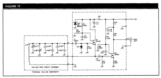
BFO oscillator and tank circuit assembly schematic.
