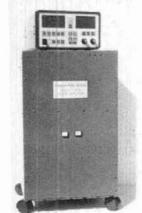
Frequency: all amateur (1.8 - 21 MHz) Drive: 50 - 80 watts for full output Output: 1500 watts PEP Input Impedence: 50 ohms unbalanced Input VSWR: 1.5:1 (higher on WARC) Output Impedence: 50 ohms unbalanced Harmonic Supp: greater than -45 dB Intermod prods: more than -35 dB down Duty: CCS (cont. commercial svc.) Tubes: EIMAC 3CX800A7 (two) ALC: 0 to -6 VDC Output Configuration: Pi-L
