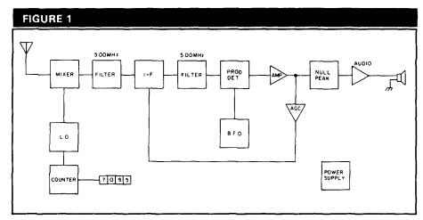
Complete block diagram of the receiver.
