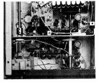
Partial bottom view showing location of switch S-1-G, input attenuator board, crystal-calibrator board, and oscillator board.
