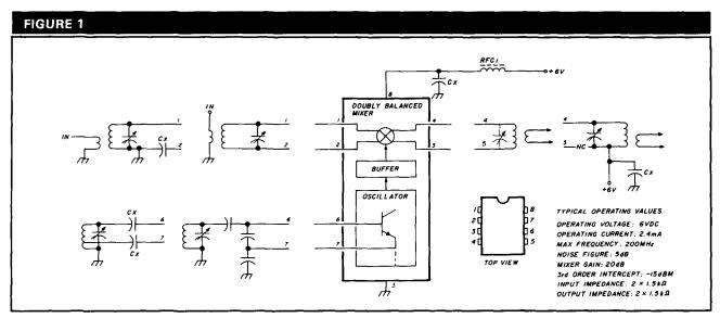
One of the possible configurations of the NE602N. Balanced circuits are preferred, but may be difficult to implement. Cx: Blocking/bypass capacitors, 0.001 to 0.1  $\mu$ F, depending on operating frequency. RFC 1: Ferrite beads or RFC, recommended at higher frequencies.
