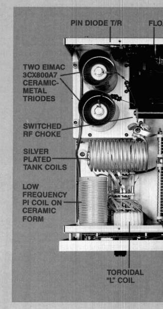
All the new **ALPHA's** use a pair of Eimac 3CX800A7 triodes to provide maximum legal power in all modes with plenty of reserve. Tuned inputs assure easy excitation to full rated output with superb linearity and efficiency.
