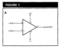
Standard op-amp symbol. The pin outs are "industry standard" 741-family and fit a large number of different devices.
