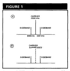
A normal AM carrier supports two sidebands, one below and one above, shown at A. Removing the carrier, as at B, leaves the sidebands, which are the elements that transmit information. After generating the sidebands, the carrier is no longer necessary for transmission.
