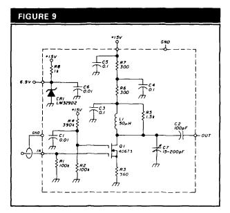
VFO buffer amplifier schematic.
