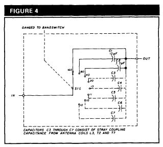
Wafer switch and coupling capacitors between antenna and RF coils.
