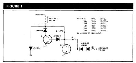
Schematic of the circuit used to interface from the +12Vdc keying output of the TS440S to the -120 volt bias supply of the Heathkit amplifier.
