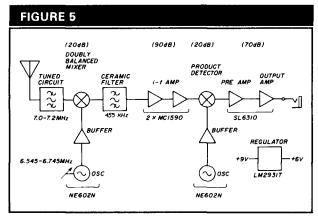
Block diagram of the  $5\times 8$  40-meter superhet receiver. There are ten functional stages in five 8-pin ICs.
