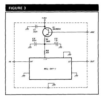
Input attenuator schematic.
