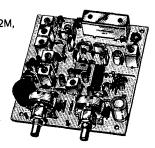
•R451 UHF FM RCVR. Similar to above. Tuned line front end, 0.25uV sens. (0.1uV with optional hel. res. preamp). Kit \$149, w/t \$229.
