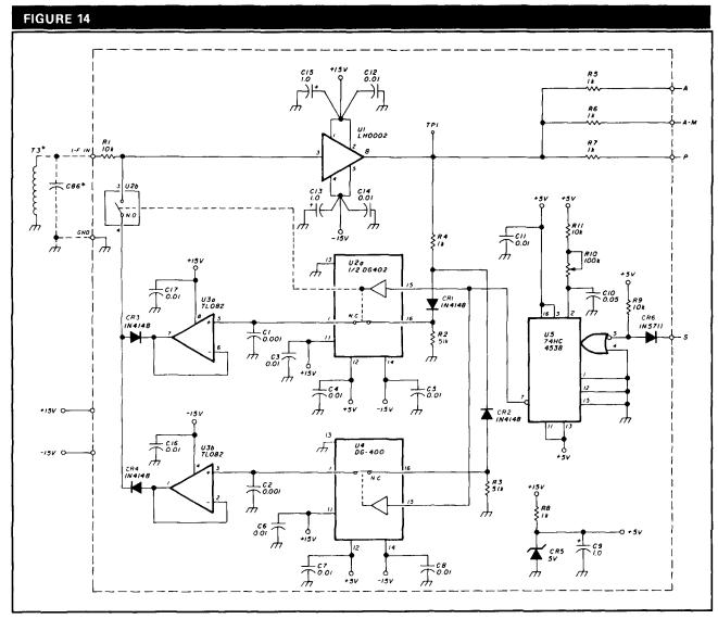
I-F buffer and gated noise limiter schematic.
