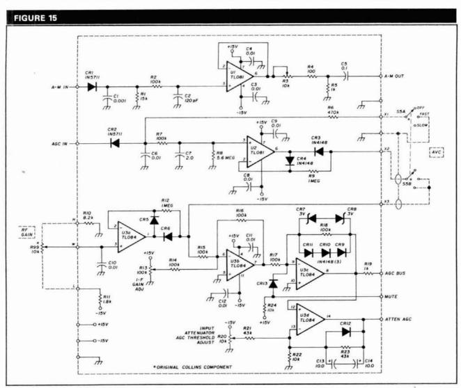
AM detector and AGC amplifier schematic.
