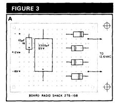
Power supply parts placement guide.
