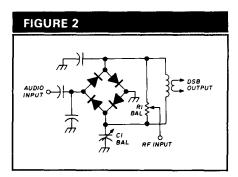
A simplified balanced modulator circuit. The RF carrier does not appear at the output, but the products of modulation — sidebands — do appear.
