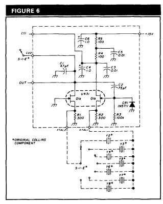
Band select crystal oscillator schematic.
