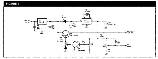
Schematic diagram of power supply/regulator.
