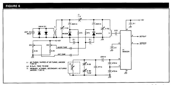
Mixer/first oscillator circuits for the  $5 \times 8$  receiver. Decimal capacitor values of  $\mu$ F; whole capacitor values are in pF. Capacitors marked /s are polystryene, silver mica, or NPO ceramic. Values are for 40 meters.
