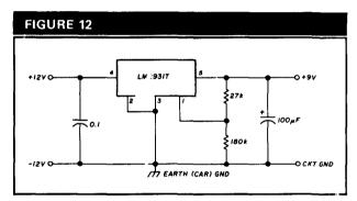
A recommended preregulator circuit for use with autonative systems or 12-volt DC wall adapters. Note that a connection to car body or earth ground is shown to reduce stray noise and signal inputs.
