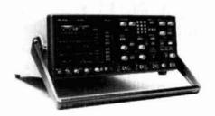
The PM 3320A DSO offers an on-board Fast Fourier Transform (FFT) option with an overview of the incoming signal's frequency spectrum. Other automatic measurement functions are: RMS voltage, percentage overshoot and preshoot for step functions, and continuously variable rise and fall times — including the two pre-set options of 10 to 90 percent and 20 to 80 percent of ECL applications. It also provides
