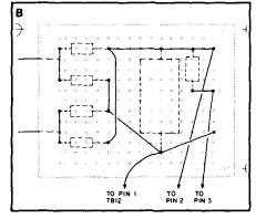
Power supply foil-side connections.
