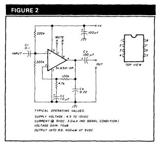
Plessey SL6310-DP high-gain audio amplifier. All capacitor values are  $\mu F$ . The values shown are for "hi-fi" operation. The low frequency response can be raised by decreasing C1, C2, and C3. The high frequency response can be decreased by increasing C4. The mute pins are internally biased, and may be left open. Grounding "A" or connecting "B" to pin 5 will mute the output. The mute connections must include a 100k series resistor.
