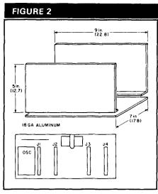
Dimensions of the receiver cabinet, and pc board placement within the cabinet.
