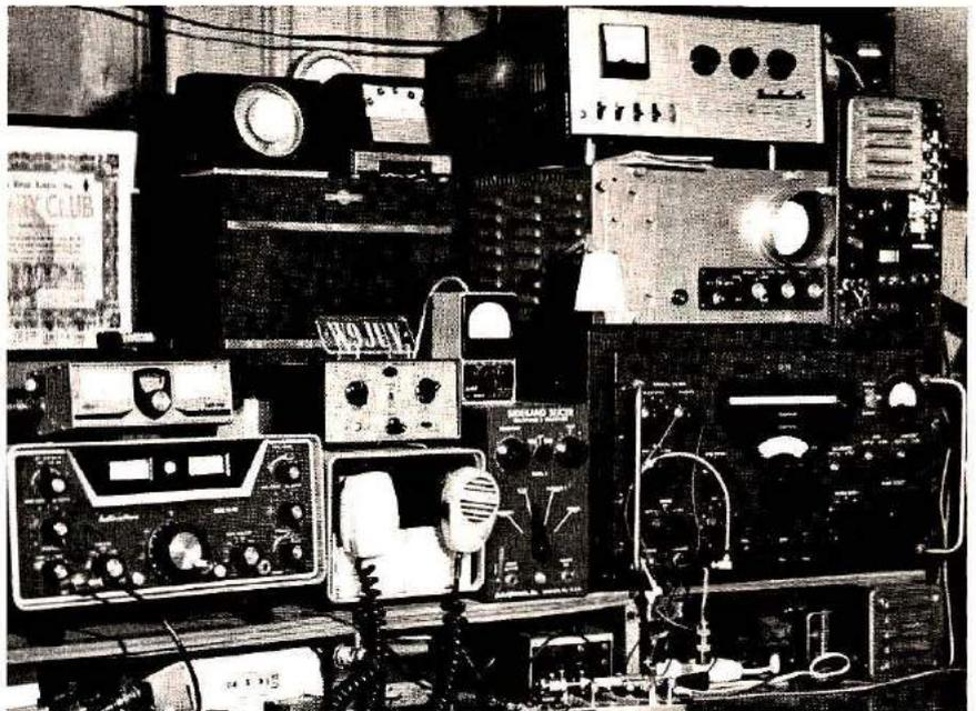
Amateurs who have been at the hobby for any length of time tend to accumulate a lot of equipment. This station includes gear for all the amateur high-frequency bands, as well as for vhf, uhf, and repeater operation. Some of the equipment is new, some is war surplus, and some is adapted from the commercial two-way radio services.
