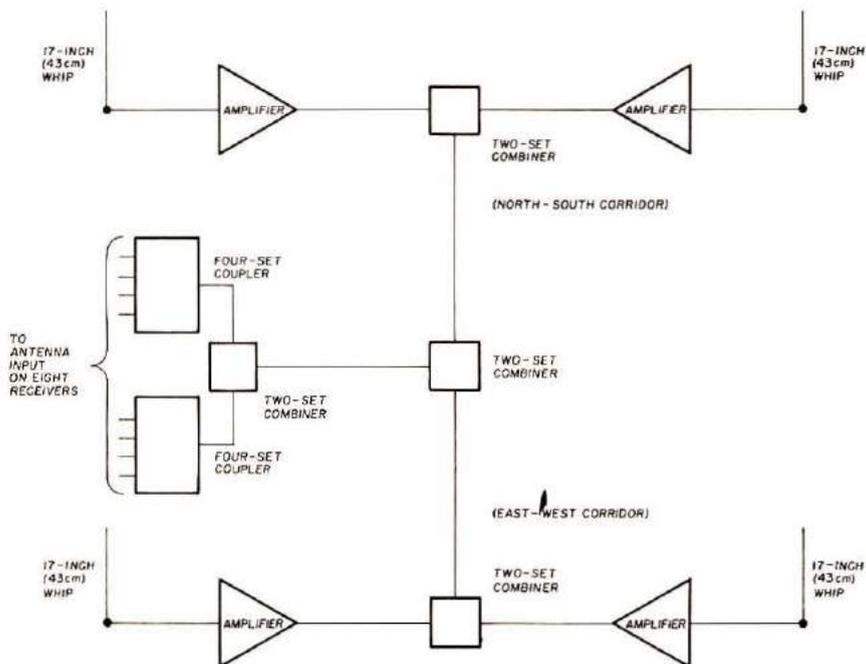
Fig. 5. Master TV antenna system components including wideband 30-dB vhf preamplifiers are used in the antenna system.
