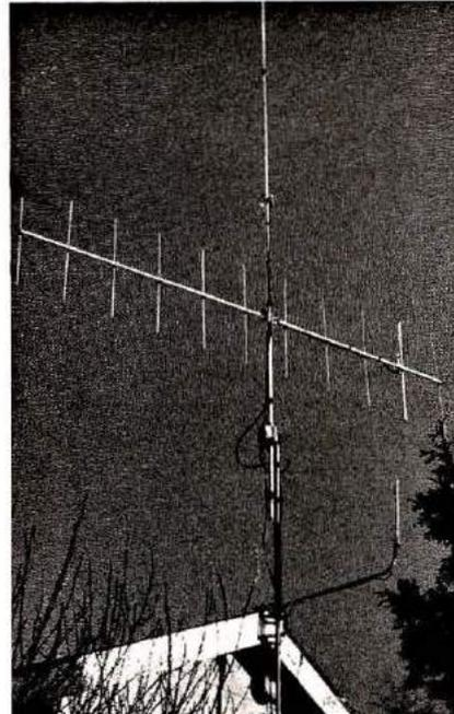
An omnidirectional antenna can be installed atop a beam, if roof space is limited, when operating two-meters. The antenna on the lower right is for the VHF (152-174 MHz) Public Service Band.
