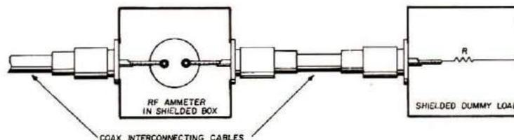
Fig. 1. A simple, neat hookup for measuring the output power of your transmitter using the dummy load described in this article. An rf ammeter is connected by coaxial cable between the antenna output terminal of your transmitter and the input terminal of the dummy load. The text describes some do's and don'ts for power measurement.
