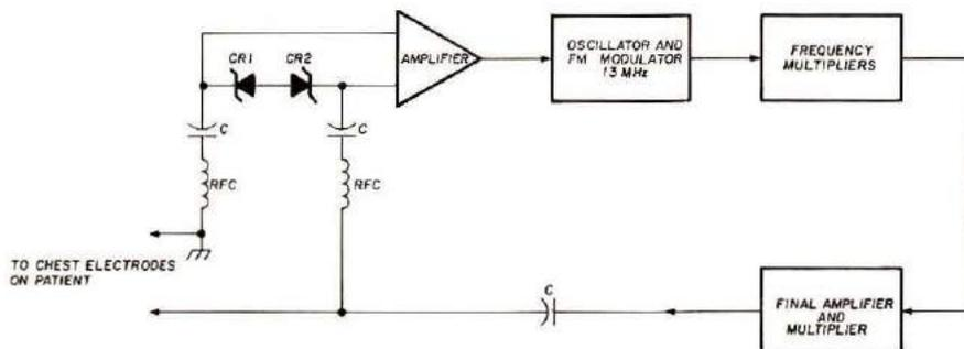
**Fig. 4.** Block diagram of a popular vhf telemetry transmitter.
