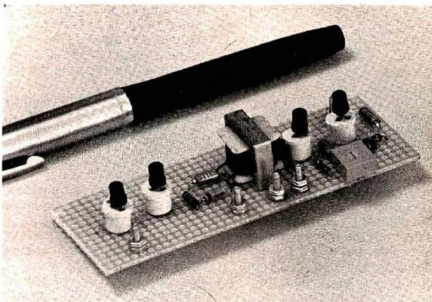
The relative size of the assembled circuit can be seen by comparison with the fountain pen. Input to the board is to the right. The small square component near the first transistor is the trimmer potentiometer to adjust sensitivity. Perforated board makes the assembly easy, and small bolts and nuts serve as connecting terminals.
