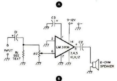
**Fig. 1.** Circuit diagram of the LM380 audio amplifier, showing the top view pin-out diagram of the LM380 at **A**, and the simple, straight forward hookup with few components at **B**. All capacitors are 25-volt electrolytic types with axial leads. The value of C1 may be between 1 and 10  $\mu\text{F}$ , C2 between 250 and 1000  $\mu\text{F}$ , and C3 between 5 and 10  $\mu\text{F}$ . R2 is the original volume control which may require an extra resistor in parallel as explained in the text.
