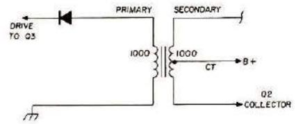
**Fig. 3.** Audio interstage transformer, T1, is connected as shown here. The primary winding is connected between diode CR1 and ground, and half of the secondary winding is connected between B+ and the collector of transistor Q2. The other half of the secondary winding is not used. Connecting the transformer as shown provides a voltage step-up.
