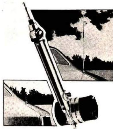
Radio Shack has just announced its new, motorized, retractable, Citizens Band antenna for mobile installations. This new antenna, marketed under the Archer brand name, can extend to its full 33-inch (84cm) length, or retract into the fender of your car, at the flip of a switch. It can be easily wired to turn the CB radio on automatically when it extends, or off, when it retracts.
