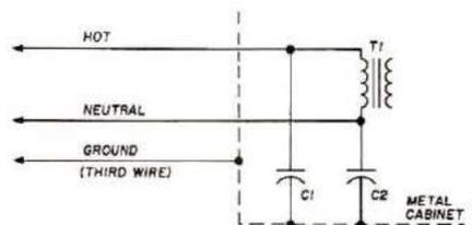
**Fig. 1.** Simplified drawing of power wiring in most electronic equipment. Capacitance between the power wiring and chassis couples a tiny leakage current onto the cabinet. Normally harmless, this current becomes dangerous if allowed to exceed 10 microamperes not passing down the ground wire.
