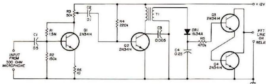
Fig. 1. The vox-box circuit is simple and requires only a few inexpensive parts. Wiring is non-critical. T1 is a small transistor interstage transformer, 1000-ohm primary, with a secondary of either 1000 or 2000 ohms, center tapped.
