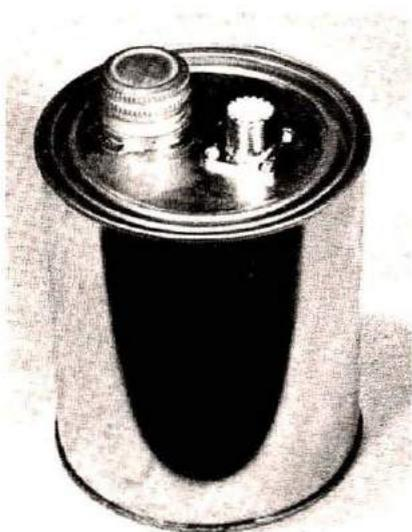
A group of resistors are immersed in oil in a paint can to make a convenient rf load for transmitter tune up. A screw-top cap from a discarded can has been soldered to the lid to allow ease in filling the assembly with cooling oil, and to provide pressure relief.
