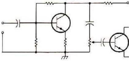
**Fig. 2.** An audio volume control may be connected as shown here, but requires two more components than the arrangement shown in Fig. 1.
