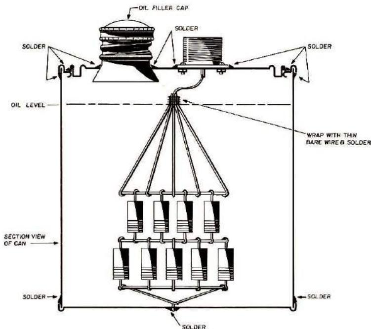
**Fig. 3.** Cross-sectional view of the completed dummy load showing details of assembly. Note the cone of wires used to connect the top of the upper resistor stack to the rf connector mounted in the lid of the can. This arrangement keeps inductance to a minimum. All seams must be soldered well, and a small air space left above the oil level permits expansion of the oil due to heating of the resistors.
