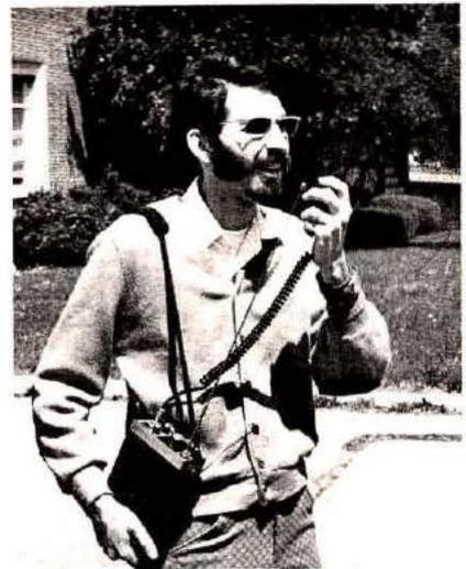
Even when he is walking, an amateur can extend the range of a 2- to 5-watt portable transceiver by taking advantage of a repeater a few miles away. This feature not only adds to the pleasure of casual hamming, but also helps in emergency situations where it is impossible to reach the scene except on foot (photo courtesy R. L. Drake Co.).
