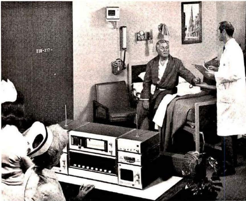
**Fig. 3.** A radio telemetry unit allows the patient to walk around a designated area while nurses monitor his ECG waveform on a receiver at the central nurses' station (photo courtesy Hewlett-Packard).
