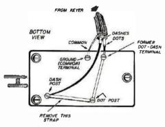
Fig. 1. The modification of a semi-automatic "bug" is started by removing the connecting strap between the dash post and the dot post. Cable from the electronic keyer is connected as shown.
