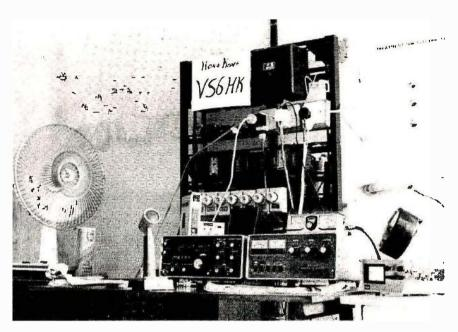
The essentials, but not much more. A Yaesu FT201 transceiver, FL-2100B linear amplifier, power/SWR meter, antenna rotor control box, and some transformers and fuses for the ac-power system take up the most of our desk top. The fan, of course, is a must-
