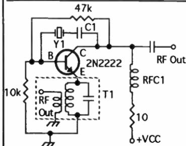
Figure 3: Bipolar crystal oscillator with tuned emitter
