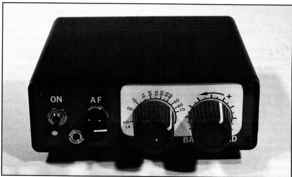
This three-IC. superhet receiver for the 20M band is about as simple and inexpensive a receiver that you can find. While it is a no frills receiver, it offers excellent performance. It is a straightforward single-conversion superheterodyne receiver for reception of SSB and CW signals. The circuit was designed by K6LMN and the printed circuit board was designed by KB6NQ.
