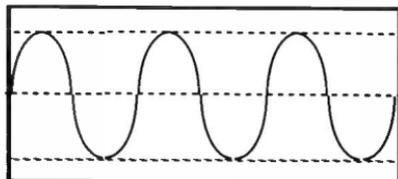
Figure 4: Output waveform of tuned-emitter oscillator
