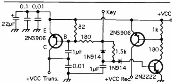
Figure 6: Transmitter keying circuit with receiver control
