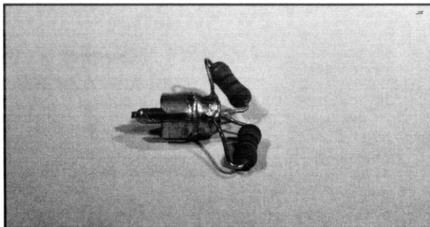
*50Ω dummy load: two parallel 100Ω, 1 watt metal-oxide resistors will handle 2 watts continuously or 12 1/2 watts for a couple of seconds.*
