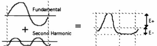
Fig. 5: Even-Order Harmonics Cause Unequal Positive and Negative Peaks
