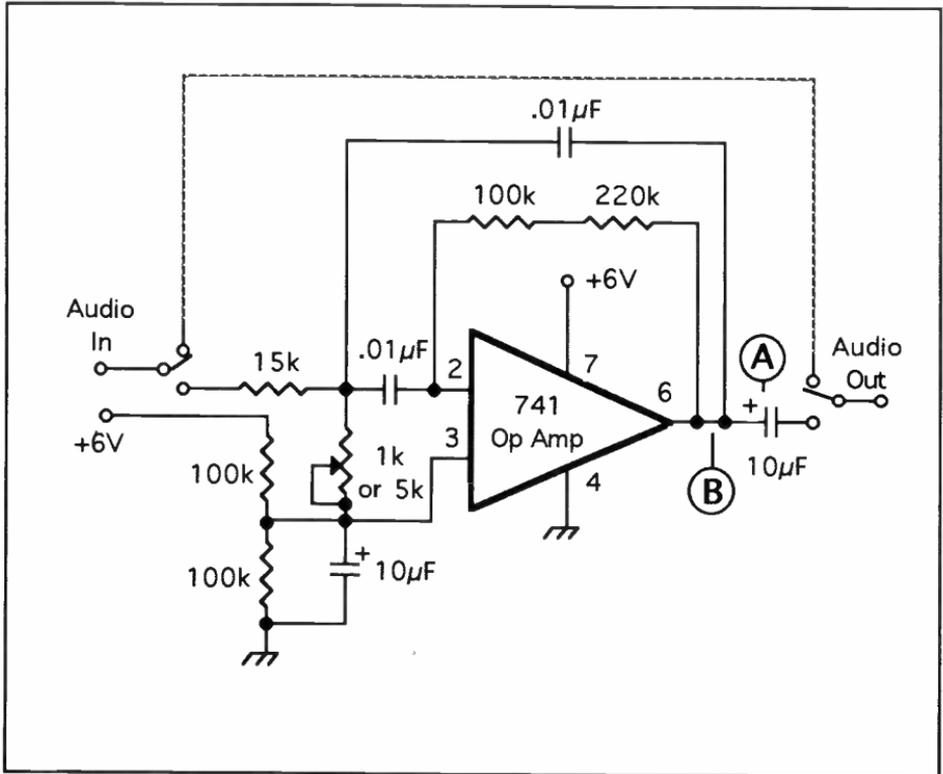
This version of the filter will play much better. Note polarity of coupling capacitor (A) and tie in of feedback capacitor and resistors (B) from pin 2 to pin 6.
