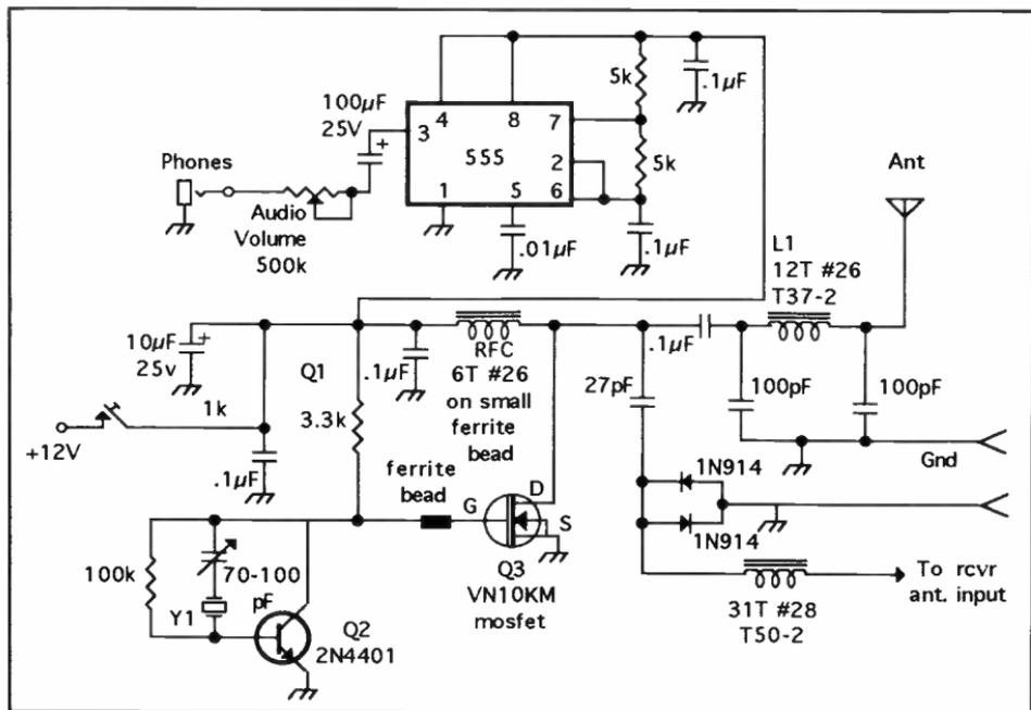
Depending on how the 70-100pF variable capacitor (in series with Y1) is tuned, the OneDer can indeed be found to chirp (at least on the *Hambrew*-built version). If this is found to be a problem, above are two mods which need to be implemented to the original schematic.
