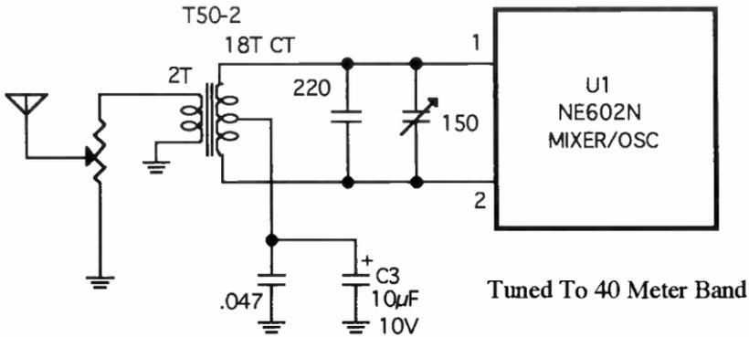
This revision reduces (but does not eliminate) AM broadcast station pickup. I believe the reduction is due to the balanced input, but it might be due to the new High-Q input circuit.
