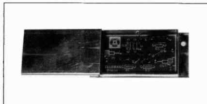
Do away with noisy signals! The K2622 gives you 22dB gain where it's needed. DC supply direct or via the coax cable (50-75 Ohm impedance), metal box included.
