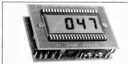
This kit provides an easy-to-read display. Because of the simple power supply requirement and compact size of the kit, it can easily be incorporated into a variety of applications.
