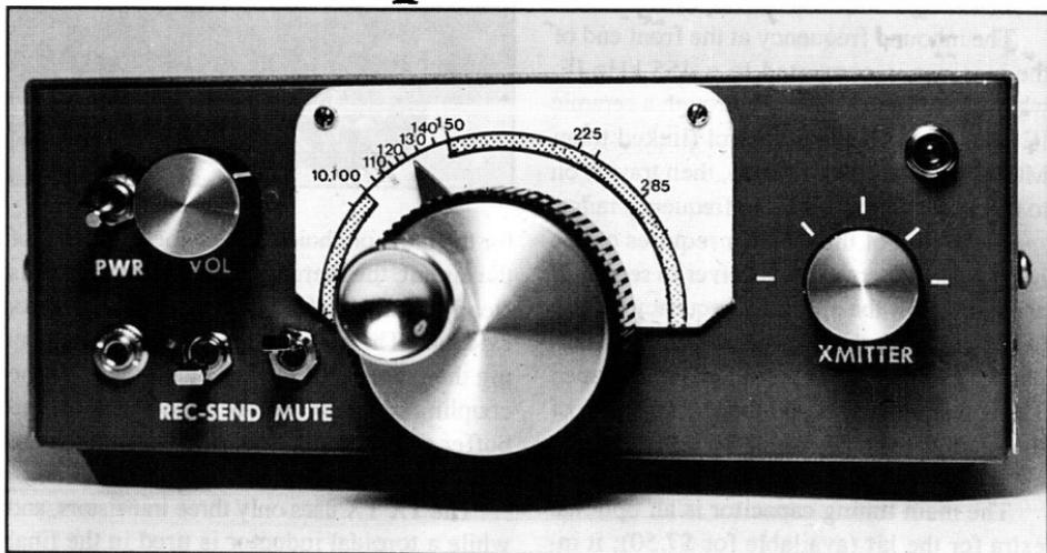
*The SupeRX/TX, available for 80, 40, 30 or 20m, includes circuit board and board components (see text).*
