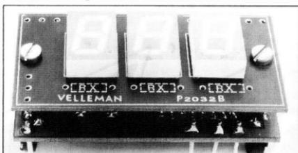
Power supply: 5VDC, 250 mA (regulated) \* Read out: -999 mV to +99 mV, 1mV resolution \* Overload indication (positive and negative) \* Linearity 0.1% \* Input impedance: 100 mohm.
