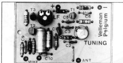
Mini FM transmitter (100-108 MHz). Integrated pre-amplifier (sensitivity 5 mV), to which any type of microphone may be connected. Power supply: 9-12 VDC.
