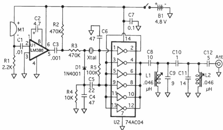
Figure 1: Circuit Diagram
