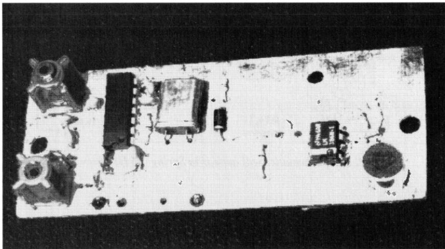
*Circuit Board: Major components (left to right) are coils, 74AC04, Crystal, 1N4001 Diode, LM386 and microphone. This board was assembled with C1 and C12 on the "circuit" side.*
