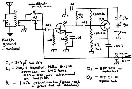
The circuit is a little unorthodox with its impedance mismatch between L<sub>1</sub> and the gate of the FET, but this helps to keep amplification down and more easily allows switching between the straight antenna tuner and the amplifier.
