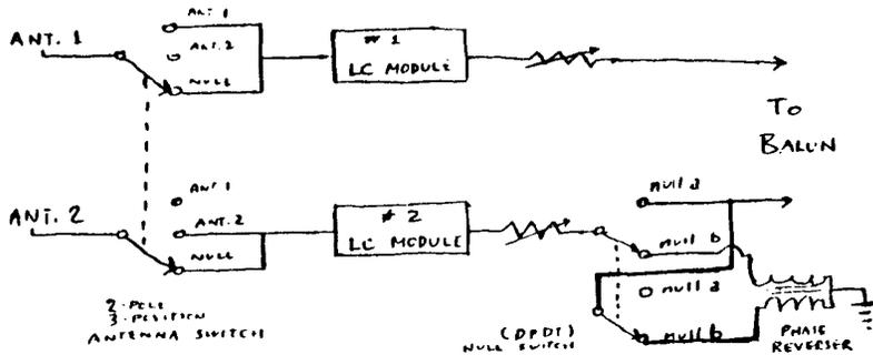
If you wanted to keep to one-switch operation while improving isolation, the 4-pole 4-position switch could be wired-in as in Figure 6.
