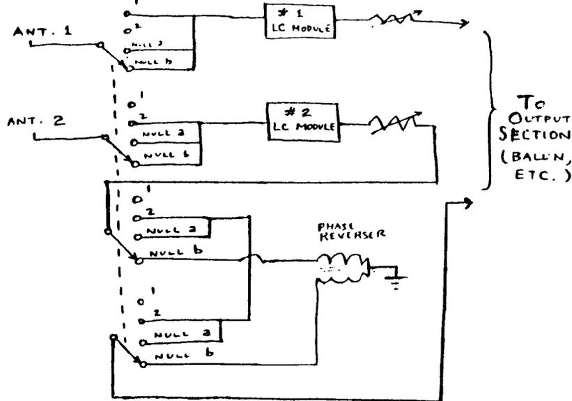
(c) Conventional phasing unit has no provision for unbalanced output.
