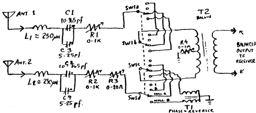
The phase-reversing transformer and the balun are wound on toroidal cores such as J. W. Miller #F-125-1, F-87-1, or T-106-2. Coil winding details will be supplied in a subsequent construction article.
