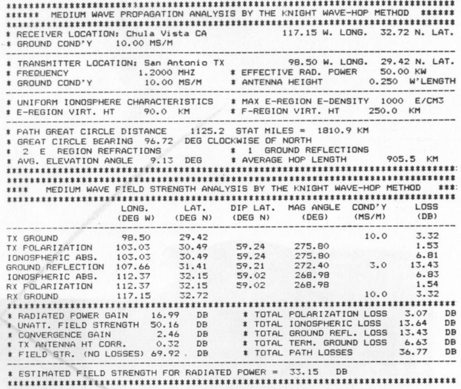
FIGURE 3. MEDIUM WAVE FIELD STRENGTH ANALYSIS - WOAI-1200 KHZ TO CHULA VISTA, TWO HOP PATH.
