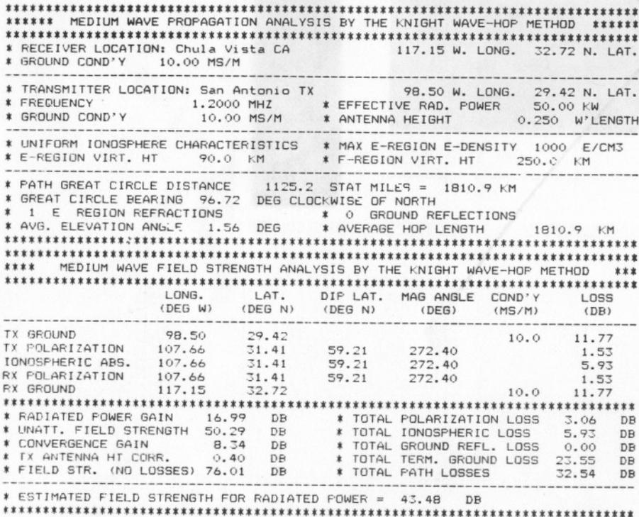
FIGURE 2. MEDIUM WAVE FIELD STRENGTH ANALYSIS - WOAI-1200 KHZ TO CHULA VISTA, ONE-HOP PATH.
