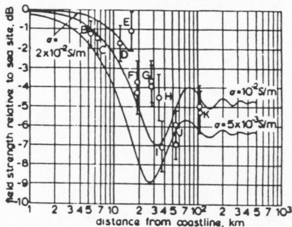
FIGURE 6. Comparison of Theoretical and Measured Ground Loss (Rome-845 Path)
