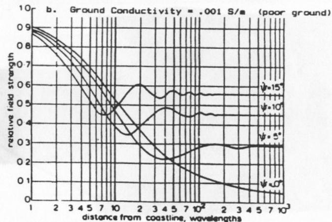
FIGURE 4. Variation of Field Strength with Distance from a Coast (Frequency = 1000 kHz)
