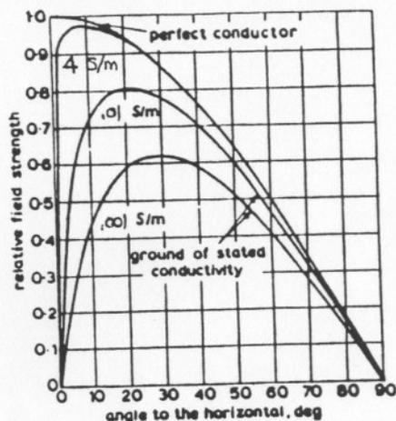
FIGURE 2. Vertical Radiation Patterns and Ground Loss for Short Antennas (Frequency = 1000 kHz)
