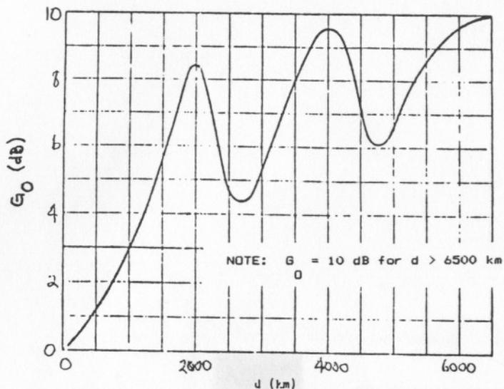
FIGURE 7. Sea Gain ( $G_0$ ) for a Single Terminal on the Coast
