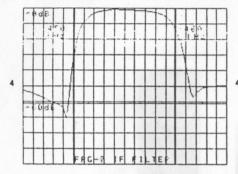
The first graph shows the Collins filter. It's center frequency is about 457KHz. It measured 3.3KHz wide at 6dB and 4.4KHz wide at 60dB. This gives a shape factor of 1:1.33. It has an stop-band rejection of 87dB. This is an outstanding measurement.
