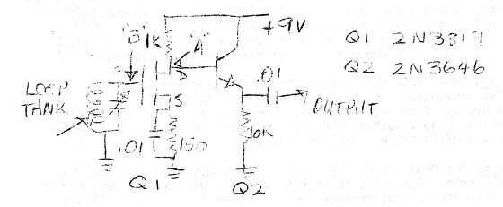
Point "B" is the input. Here, the impedance is quite high...(so am I at this point, it's 90 outside!) point "B" can be connected to the loop tank coil, or if a seperate output turn is used, to it. Either way, tuning is quite sharp. At point "B" an .01 capacitor can be placed instead of Q2 if your rx has a high input impedance. If you have a low Z input, transistor Q2 should be left in, as it is an impedance matching device, and has around 26 ohms output, with a gain less than 1.
