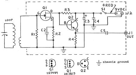
Although the circuit was originally designed for a direct coupled loop (it worked fine with a ferrite loop I threw together), it tended to overload Phil's receiver when he direct coupled it to his Wedge loop. So he hooked it up to the link coupling from his Wedge instead (as shown). This circuit was put together using perf-board and pins, and enclosed in a metal box.
