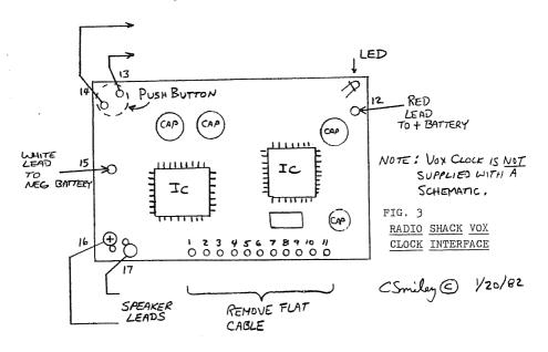
Before building this circuit, the flat flex-cable attached to the Vox Clock circuit board should be removed with care using de-soldering braid (Radio Shack #64-2090) and an iron of 30 watts or less. Three momentary push buttons with normally open contacts, such as Radio Shack #275-1571 are used for panel mounted set controls.
