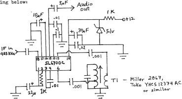
Although the manufacturer claims a possible gain of over 90 dB (!) from IF input to audio output in this IC, I didn't need all that gain. So I ignored the balanced modulator in the IC, which can be used as a linear amplifier if all possible gain is desired at one IF frequency (this device can also
