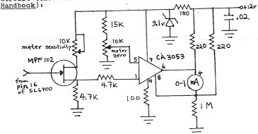
The "meter zero" trimpot is used to set the meter at zero when no signal is coming in, while the "meter sensitivity" trimpot sets the meter at its maximum reading when you local is tuned in.
