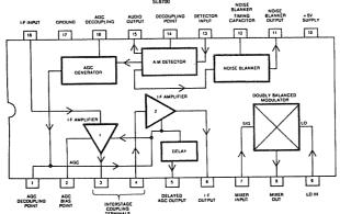
Sounds like the answer to a receiver designer's prayer, and to a large degree it is. The SL6700 was featured in a receiver description article in QST of April 1981, and I took the circuit in that article, and combined it with a circuit described in the IC's spec sheet to come up with the wiring below:
