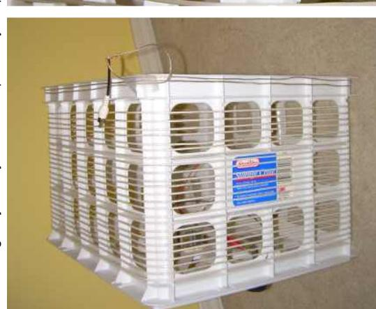
While some loop designs call for the sense coil to be wrapped in the middle of the main coil, this is too close here, and can be confirmed by holding an Ultralight receiver right up next to the main coil –
