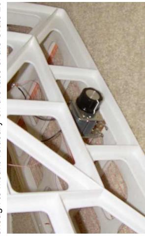
you should find the tuning sharpness of the Crate Loop to be degraded and the signal transfer decreased. By pulling the receiver away a couple inches, the tuning sharpness and signal transfer are both improved. Fortunately, my crate had a natural sense winding channel at the far edge, a couple inches away from the coil.
