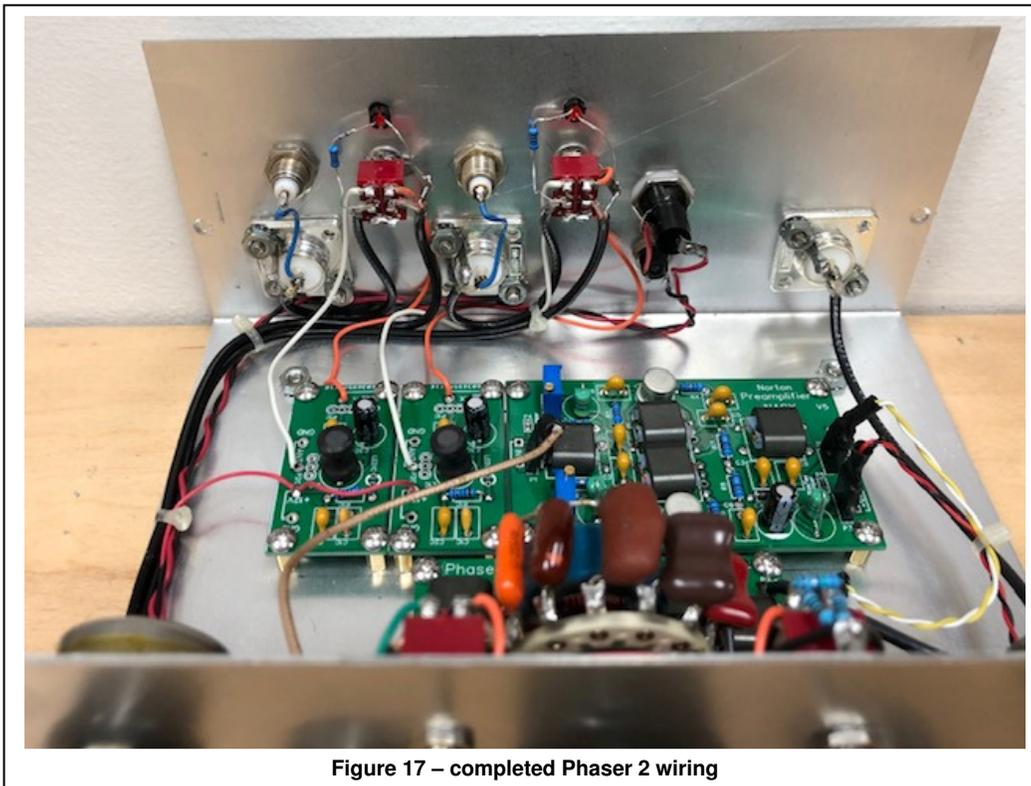
**Figure 17 – completed Phaser 2 wiring**
