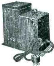
With this device you CAN BE SURE that your receiver will bring in EVERY STATION that is capable of PICKING UP, WITHOUT MISSING OR SKIPPING. Snapping a toggle is the entire operation. When switch is ON, the receiver will emit a whistle every time it is tuned to a station. Snap switch OFF, whistle disappears and station remains at peak . . . No tampering with wiring of receiver to install. Uses one tube powered from receiver. Formerly sold for \$6.75 less tubes.
