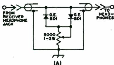
Fig. 3. audio clipper for high impedance input
