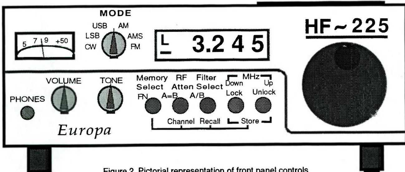
Figure 2. Pictorial representation of front panel controls
