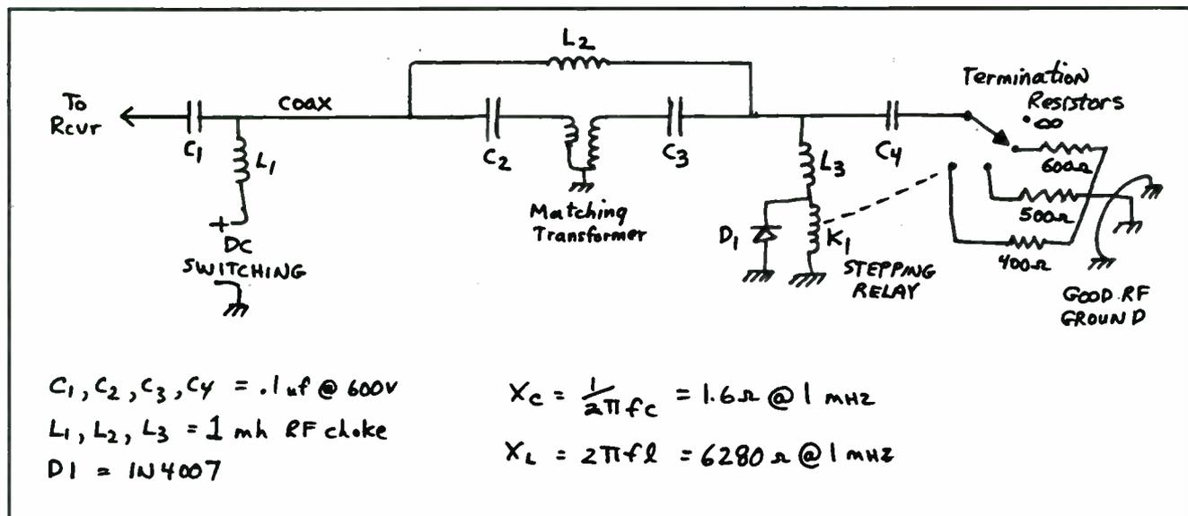
Figure 3. Basic DC switching and isolation techniques
