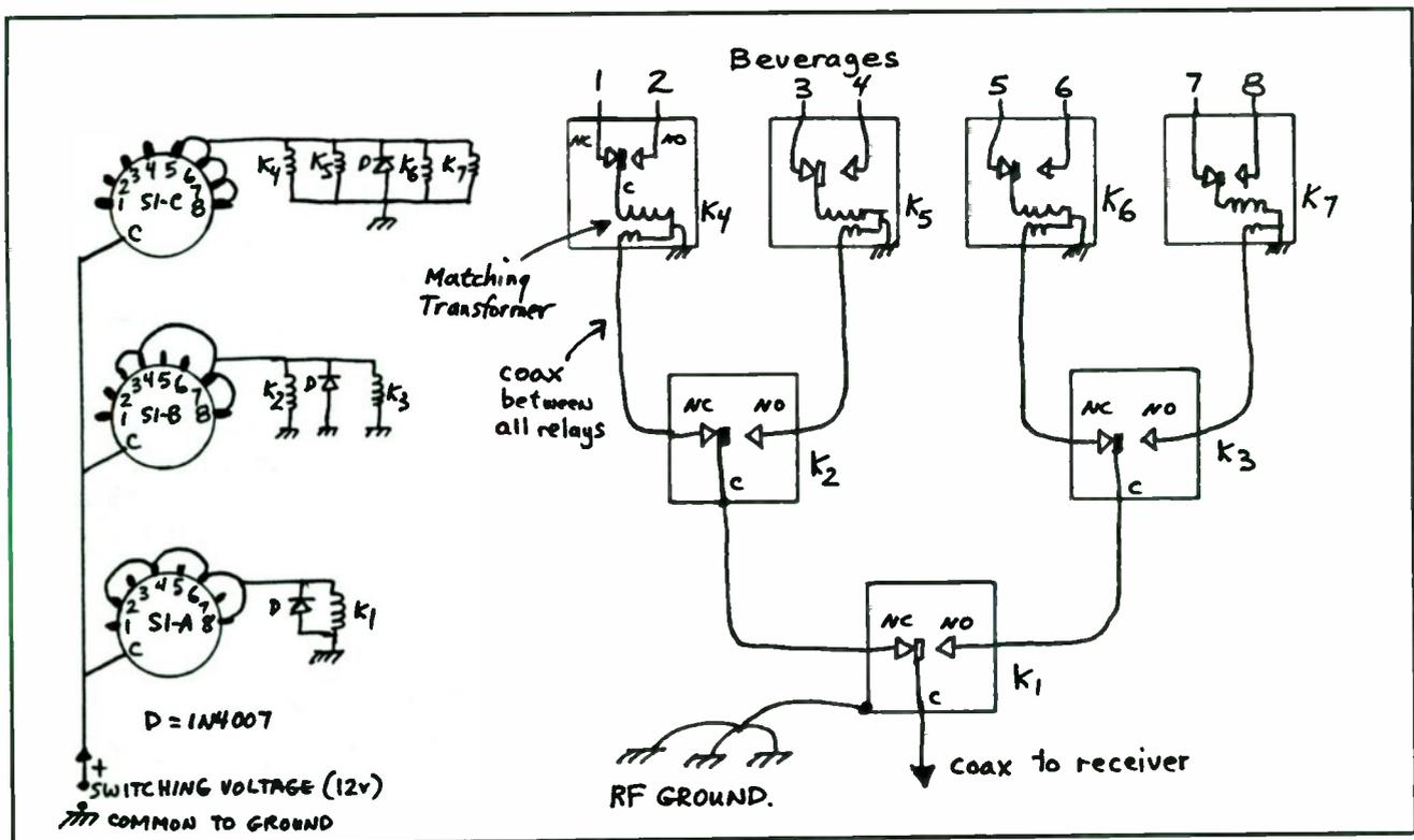
Figure 2. Switching 8 antennas using 3 control wires
