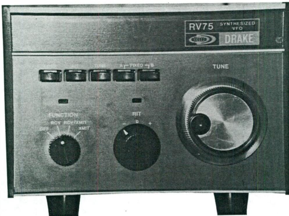
Figure 3: Front Panel Close-up of RV75 Remote VFO
