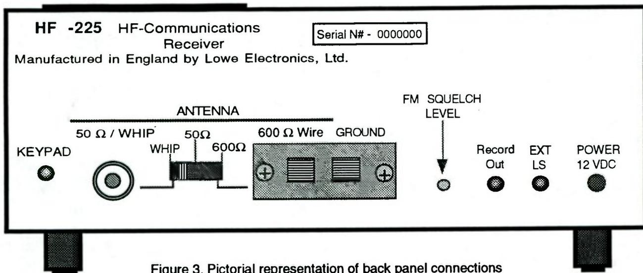
Figure 3. Pictorial representation of back panel connections
