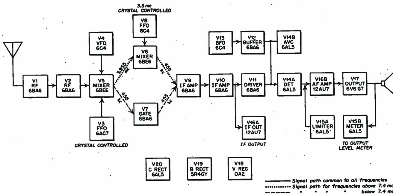
Figure 3: SP-600-JX-17 Block Diagram
