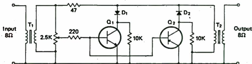
Fig. 4. audio clipper for low impedance input
