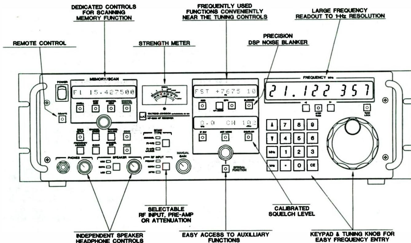
FIGURE 3. HF-1000 FRONT PANEL LAYOUT AND FEATURES
