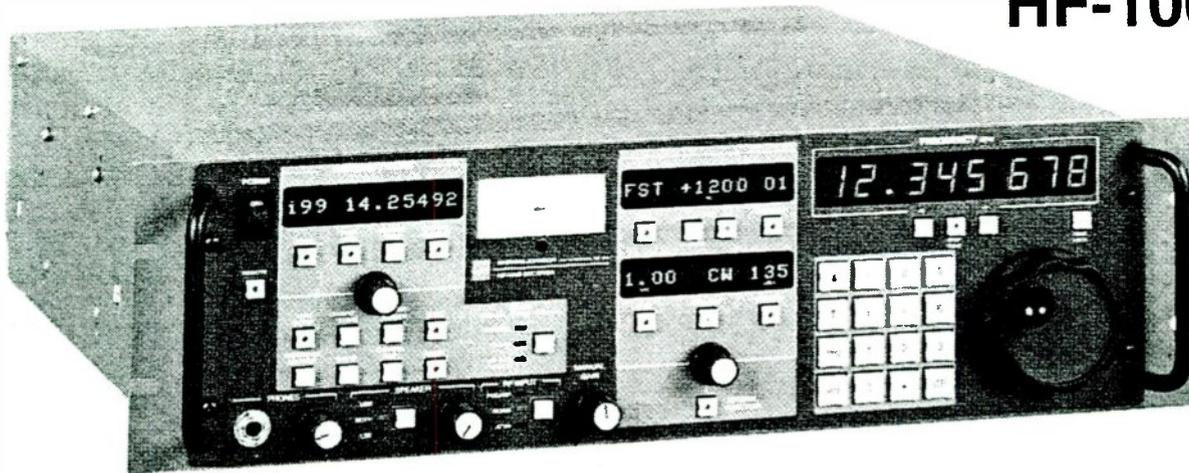
Figure 1. MODEL HF-1000 GENERAL COVERAGE RECEIVER
