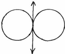
Normal Undistorted cosine loop pattern; nulls exactly  $180^\circ$  apart.
