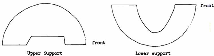
The supports are fastened inside the housing pipe with #6 x 1/2" sheet metal screws. Locate them 5 inches from the center of the tube, the upper and lower supports going respectively into the top and bottom sections of the housing. Use 3 screws in each support. Next, make the elevation yoke. Cut the following parts from 1/4" plywood, (see next page)
