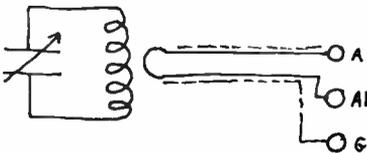
Figure 2. Balanced feed-line: double coax or shielded two conductor mic cable. Connect one conductor to "A" terminal on receiver, and the other to "A1". Shielding is connected to the ground terminal.
