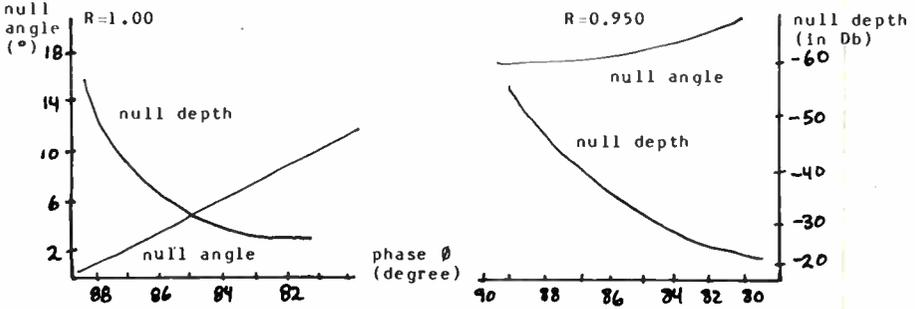
In the first case we set the pickup ratio,  $R$ , exactly equal to 1.00 and let the phase drift by a few degrees. Note that the nulls drift apart somewhat but, more significant, the null depth is very seriously affected - only a two degree error in setting the relative phase degrades the nulls so severely that they are only 35 db deep.
