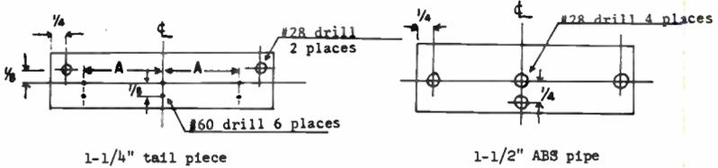
(For pipe length of 2-7/8", Dimension "A" is 3/8 inch. For pipe length of 4-1/2", Dimension "A" is 1-13/16 inch and for 8-7/8 length, "A" is 4 inches.)
