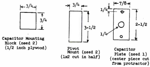
Assemble the parts as shown in the photographs and following diagram. The housing is fastened to the yoke spacer with three #6 x 1" sheet metal screws. All other parts are glued together, except for the capacitor mounting plate which is mounted with two #4 x 1/2" sheet metal screws. The FET preamp is mounted to the elevation yoke with two #6 x 1/2 inch sheet metal screws. Refer to the diagrams below.
