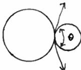
"Skewed" loop pattern; nulls are separated by  $\theta$  degrees; in a pattern controlled loop this angle could be altered at will.
