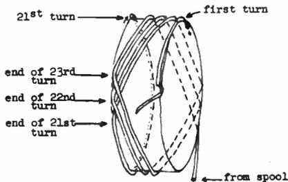
Universal Wind showing  $1/4$  of first, and  $3/4$  of last solenoid turns; and  $2\frac{1}{2}$  turns of Universal winding.
