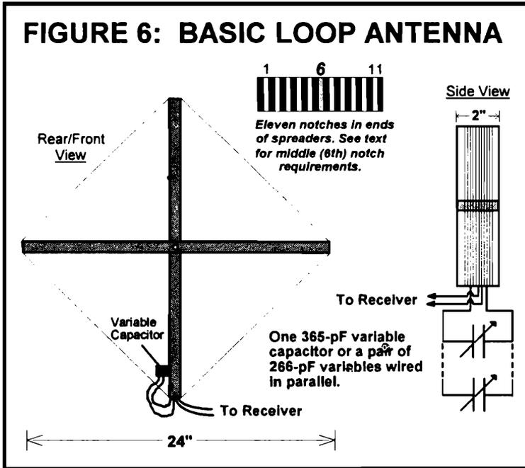
Along the width of the four edges of the spreaders make 11 notches spaced about 1/8" apart. These grooves will allow the wire to sit uniformly when you form the loop. On the bottom spreader, nail in one small nail each at the first and last (eleventh) notch. Also at the middle (sixth) notch, nail in two small tacks. These tacks will serve as fastening points for the wire you are about to wind.
