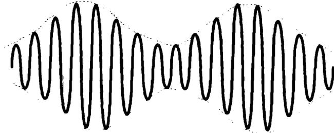
B. Amplitude modulated (AM) RF carrier wave
