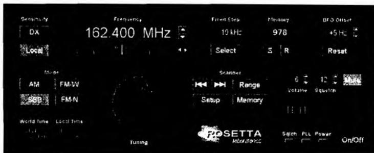
**WinRadio is a 500 kHz-1300 MHz scanning receiver on a PC/AT computer card controlled by software**
