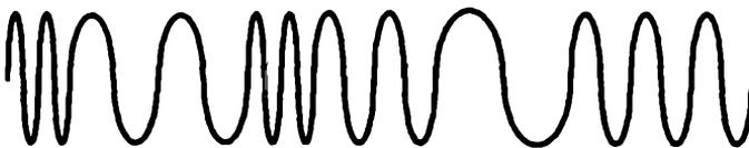
C. Frequency modulated (FM) RF carrier wave
