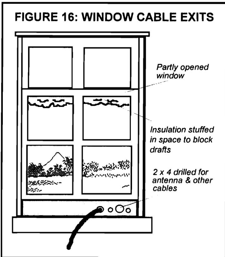
A common 2" x 4" board can be cut to fit a window. Drill holes to allow wires to pass. This is a good temporary setup until you decide on a permanent scheme for your monitoring post. Some people replace a pane of glass with Plexiglas or acrylic. This lets you make holes and still keep the window fully closed.
