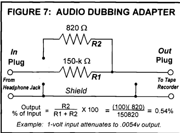
All you need to do to make your own cable is to wire a 150 kΩ resistor into the center conductor of the shielded cable and a 820 ohm resistor from the shield to the center conductor. You may have
