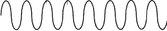
A. Unmodulated RF carrier wave
