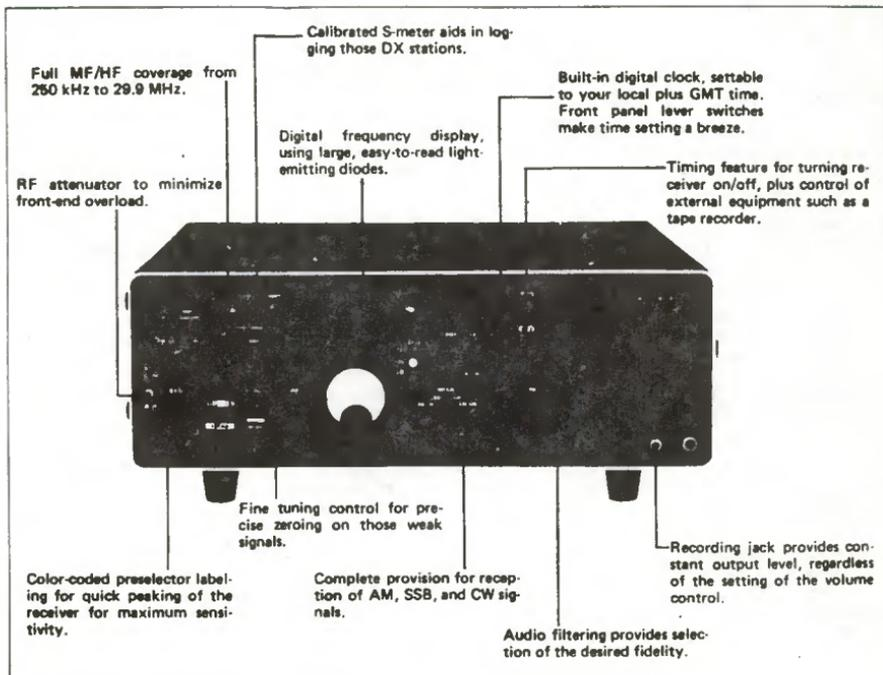
The FRG-7000 has a rugged metal case with feet on the bottom and on one side. On the side opposite the feet, there is a carrying handle so the receiver can be handled like a piece of luggage. The front feet on the bottom are longer so that the receiver sits at a convenient angle. The receiver has its own front panel speaker.
