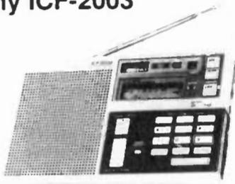
The ICF-2003 covers 153 - 29995 KHz and FM. A BFO is provided for SSB and CW. Advanced features include: LCD digital readout, keypad entry, ten memories, scan, 12-24 hour clock-timer, LED tuning meter and tone switch. With earphone, carry case, battery case, AN 6 wind-up antenna and SW guide. Requires six AA cells (not supplied).
