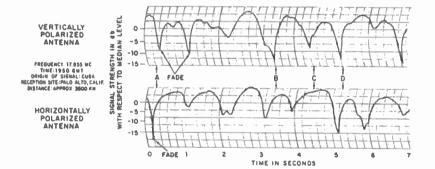
Figure 1 Vertical and horizontal components of signals from Radio Havana Cuba, as received in California, are anti-correlated.
