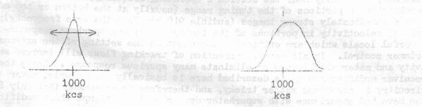
Figure 1 (a): most good receivers have an antenna trimmer control to allow the operator to bring the antenna stage resonant frequency exactly to the signal frequency, in this case, 1000 kcs. AT is the antenna trimmer. an external control.
