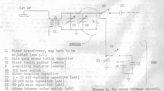
and shielding of the mixer and oscillator circuits; careless placement of this additional circuitry, simple though it may be, can inadvertantly thwart this isolation and result in extreme instability, spurious oscillations, etc. In the relatively unlikely event that problems of this nature arise, previous experience with superhet circuitry may prove very useful.
