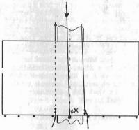
If the FET's are not used, wind an 8 turn tank instead; pass through hole in Al after 4 turns have been added. The link coil consists of 2 turns as shown above; the ends are anchored through the holes near the center of the plate.
