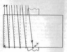
After 5 complete turns have been added, the wire passes through the hole drilled through arm Al; winding then continues as before until a total of 10 turns have been made. Pass end of winding through the pair of holes on right side of plate to anchor. Strip insulation away at point "x" for center tap. Spacing between adjacent turns should be made exactly one-half inch!
