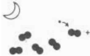
At night the free electrons recombine with the gas and the amount of MW signal absorption falls off rapidly.
