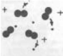
Sunlight causes electrons to be stripped from gas molecules and these free electrons absorb MW.
