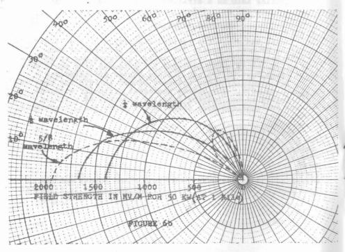
A. For the quarter wavelength antenna shown on 6a, what is the expected radiation level encountered 40° above the horizon, 1 mile from the antenna?
