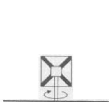
The horizontal pickup pattern for a loop antenna describes what happens to the signal strength as the antenna is rotated. Signals are strongest when the plane of the loop points at the station; the null (or minimum pickup) occurs when the station is broadside to the plane of the loop.
