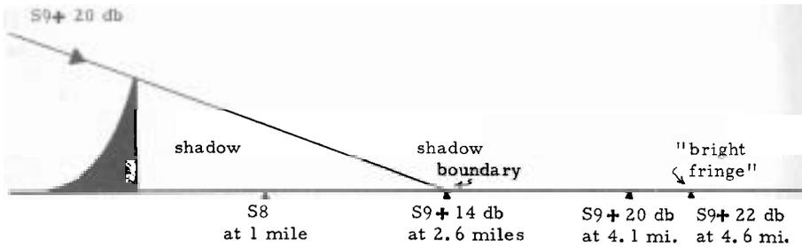
Figure 4. The arrival angle of the signal is 20° and the assumed strength is S9+20 db were the mountain removed.
