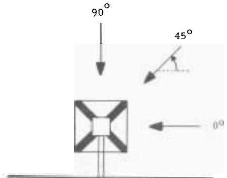
The vertical pickup pattern of a loop describes how much signal is picked up for different signal arrival angles above the ground beneath the antenna. If the signal arrives parallel to the ground (the lowest possible skywave signal), the arrival angle is 0° and the loop exhibits maximum sensitivity. As skywaves arrive from higher and higher angles the pickup of the loop falls off steadily.
