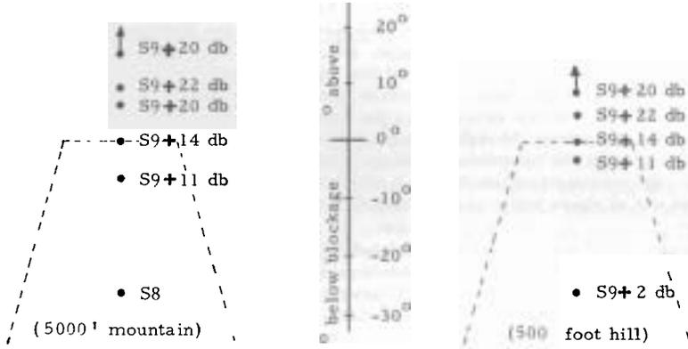
Figure 6. Horizon blockage diagrams taking diffraction into account. The incoming signal arrives at 20°; the above diagrams show the amount of signal audible due to diffraction at different receiving site locations. The 0° point is the shadow boundary at 2.6 miles.
