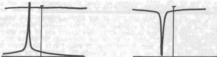
Fig. 11. (a) (theoretical curves). Theoretical flat mixer band-pass with Q-Mult off, and the shape of the Q-Mult Peak function curve is shown, illustrating no gain except at the peak frequency. Drawn to fit coordinates of the SB-620 screen.
