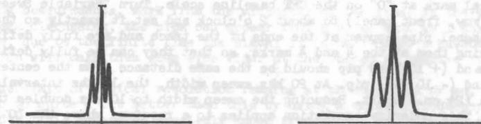
Fig. 9. (a) Sidebands from a station testing with 1000 hz audio, seen with variable sweep width = 20 khz and sweep width switch set for 50khz position. (b). Same signal as at left, except the variable sweep width pot is set fully CCW, sweeping about 7 khz. Note increased resolution of sidebands.
