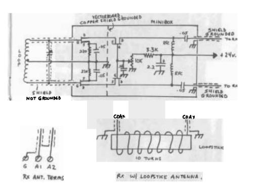
loop wire - Belden indoor antenna wire #8014
