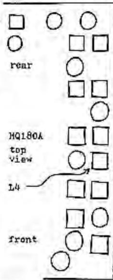
10. The RF generator is NOT connected to the junction of C28 and T5 and chassis ground, but instead is connected to pin 7 (the grid) of V2 (the first mixer). Now align the 60 kHz IF strip per the HQ180A manual. (Be sure to set your VTVM for FETVOM for negative DC readings).
