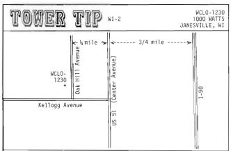
WHAT TO LOOK FOR: One self-supporting tower, lighted at night, about 200' tall with FM antenna elements side mounted at the top.
