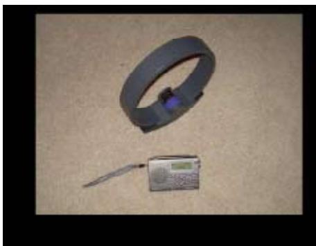
Adjacent Orientation - Quantum Loop and 15" box loop
