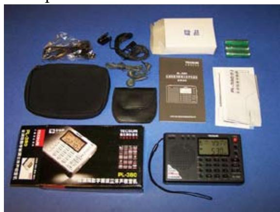
the batteries from a computer, a Chinese owner's manual and registration card, a vinyl carrying case, stereo ear bud phones and case, a clip-on wire antenna, and a wrist strap attached to the PL-380 cabinet.
