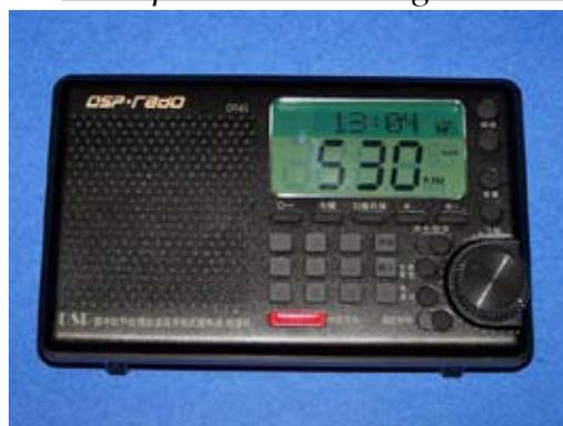
In the case of the D92L, however, the design itself had severe shortcomings, including a digital section generating RF hash to degrade AM sensitivity, and a 15-second digital “chuffing noise” whenever a control was changed. As such, the D92L models never really caught on with AM-DXers.
