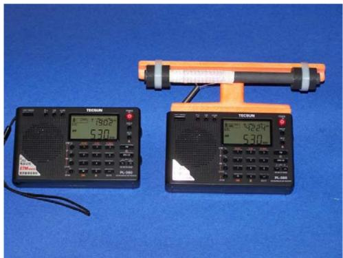
after the Slider coils were peaked. This provides an obvious advantage of allowing a DXer to chase transoceanic DX during brief band openings, without the need to peak a coil each time a new frequency is selected.
