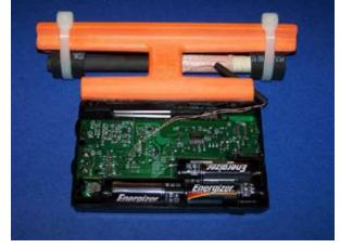
connections previously used by the stock loopstick. Place a small strip of strapping tape (insulating type only) across these newly soldered leads, and carefully mate the front and back cabinet sections together, routing the Litz wires through the empty hole left by removal of the wrist strap. Reinstall the four cabinet screws and the three AA batteries, and check for normal operation.
