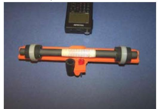
Referring to the loopstick construction section above, complete the coil winding procedure and secure your loopstick on the completed plastic frame, using the suggested rubber shock mounts to protect the ferrite bar.
