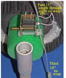
insert its end up through the right side tie wrap eye (as shown in the photo) for a length of 11", passing the tip in between the Litz wires and over the top of the variable cap, as shown
