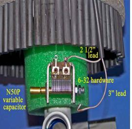
terminal shown, ensuring that there are no shorts to the variable cap frame. Prepare the end of the 3" Litz wire lead as shown, so that it will fit securely between the 6-32 nuts when the screw is tightened in a clockwise pattern.
