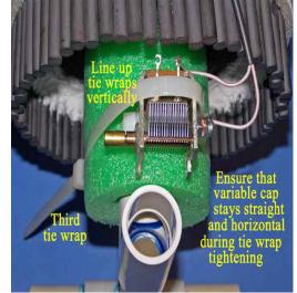
29. After the variable cap is secured tightly against the Funnoodle surface, turn the shaft of the
