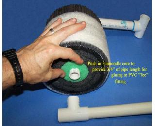
this "Tee" fitting until the end of the scrap piece of 34" PVC pipe lays on the table, to the upper right of the antenna assembly. In the same way, insert another scrap piece (12" or longer) of 3/4" PVC pipe in one side of a remaining PVC "Tee" fitting, and lay this scrap pipe in front of the antenna assembly, parallel and lined up with the scrap PVC pipe in back of the antenna assembly (refer to photo at left).
