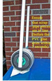
the two 4" long PVC pipes in their place (in one end of each of the two "Tee" fittings), making sure that the pipe sections are bottomed out in the "Tee" fittings, and that both 4" pipes are facing in the
