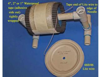
17) Refer to the photo at left for the following step. Place the FSL assembly in the position shown, and tightly wrap a turn of your wider waterproof tape around the center of the FSL assembly (adhesive side out), overlapping the ends by 2". If you are using the 1" wide waterproof tape, wrap two turns, with the edges overlapping by 1/4". Temporarily tape one side of the 660/46 Litz wire to the right side of the Noodle (as shown) with a scrap of waterproof tape.
