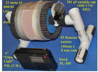
6) An FSL's DXing performance can be increased by placing the antenna on a non-conducting stand up off of a table, such as on a PVC-framed base for DXpedition or shack usage. Information on such PVC bases and a protective "rain hood" PVC assembly may be obtained from the author.
