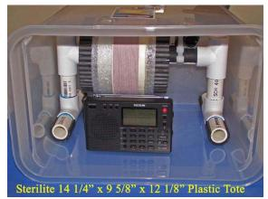
of the 45 ferrite rods. Finally, the antenna has slip-resistant rubber grips on the two PVC "legs" for operation on wet surfaces, and provisions have also been made for plugging in a protective "rain hood" assembly. A compact Sterilite plastic tote (14 ¼" x 9 5/8" x 12 1/8", which is commonly
