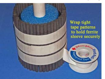
tape turns help to secure the ferrite sleeve assembly in a cylindrical shape, and should be installed immediately after completion of the ferrite rod installation.
