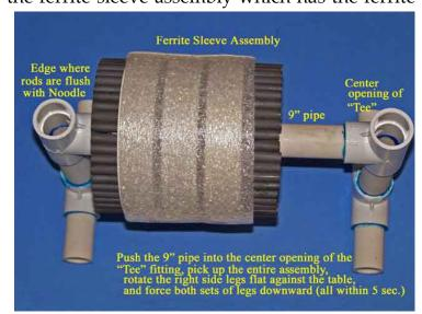
"leg" assembly so that both sets of "legs" are fairly flat against the table. Force both sides of the frame hard downward against the table until the right side "leg" assembly is perfectly straight (while the glue is still wet, putting downward pressure on both sides of the frame will provide a perfectly straight match of the "legs," as long as the table is perfectly flat). This completes the assembly of the antenna's PVC frame—allow the glue fumes to vent outdoors before proceeding
