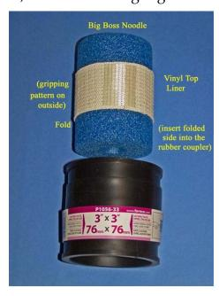
smoother side of the vinyl liner is on the inside, and the side with the gripping pattern is on the outside). Wrap this folded section as shown around the center of the Big Boss Noodle section, pulling it tightly so that one edge overlaps the other. Secure this overlapping section with a 2" strip of Scotch "Extreme" tape, as shown.
