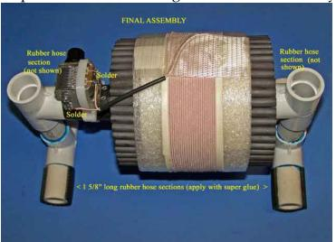
super glue has been applied, while ensuring that the borders of each rubber hose section are aligned with the edges of the PVC "legs. This completes the assembly of the 5" FSL antenna, which is now ready for testing and operation.
