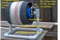
area. The quality of a signal null is also related to the FSL's design (i.e. the symmetry of its cylindrical ferrite sleeve, and the degree to which the variable cap size and variable cap wiring cause distortions in the symmetrical RF reception pattern). For the best possible pest station nulls, the use of a rotating support structure (i.e. Lazy Susan table) is recommended.
