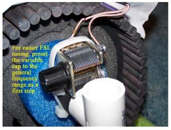
the portable radio (see photo at left). The variable cap's tuning plates can be observed to preset this approximate frequency (i.e. fully meshed for a very low band signal, half open for a mid-band signal, and close to fully open for a high-band signal), thereby saving time and effort in the next step.
