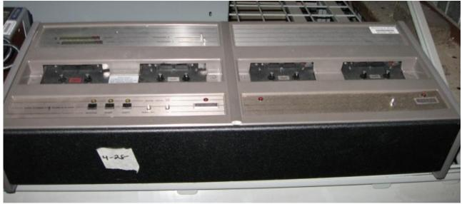
The master duplicator, (seen above), and the slave, (seen below), were "preventative maintenance serviced" in 2011, have all new belts and heads, and have been aligned and speed checked for accuracy. Both units are working.
