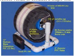
unplanned "drop tests." At 22 pounds (10 kg), this new FSL had the size, weight and feel of a DXing monster... and at a \$500 construction cost, this "Financial Sinkhole Loop" also provided a pretty scary example of the relationship between FSL price
