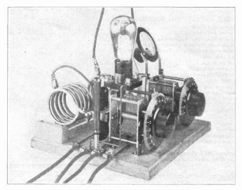
THE LOW-POWER HARTLEY TRANSMITTER The tube socket is mounted by brass angles on the rear of the tank condenser. The socket terminals should be well insulated from the supports.
