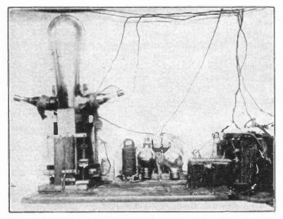
A PRACTICAL MERCURY-ARC INSTALLATION Note the framework supporting the tube and the solenoid used for tilting it by remote control.
