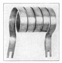
PLATE TANK INDUCTANCES for a high-power transmitter can be made in this fashion. The copper strip is  $V_8''$  thick and  $V_4''$  wide.
