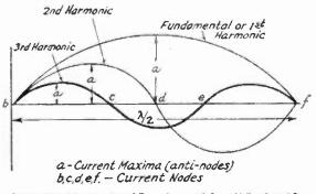
CURRENT AMPLITUDE OF 1st, 2ND, AND 3RD HARMONICS (Oscillations in a half-wave antenna)
