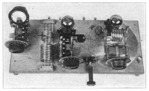
THE TRANSMITTER WITH THE OSCILLATOR SHIELD REMOVED The amplifier receives excitation through the lead tapped on the oscillator inductance. A connection is made by a clip at the center of the amplifier tank inductance. The neutralizing condenser is connected between the grid of the amplifier tube and the front terminal of the tank inductance.
