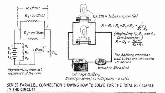
since these resistances are small in comparison with vacuum-tube and rheostat resistance. Thus it is that in the vacuum-tube circuit shown in the large diagram, the wiring and  $R_1$ ,  $R_2$  and  $R_3$ are neglected.
