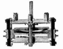
Among the special purpose condensers is the 201-E, a Taper Plate condenser, in which the stator plate is adjustable, affording maximum capacities from 50 mmfds. to 10 mmfds. with a constant minimum of 7 mmfds.
