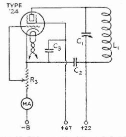
WIRING OF THE A.C. DYNATRON FREQUENCY METER
