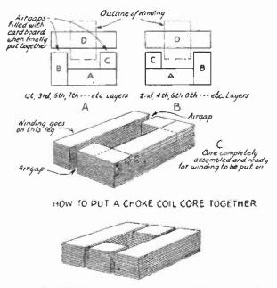
ANOTHER METHOD OF BUILDING A CORE FOR A CHOKE COIL
