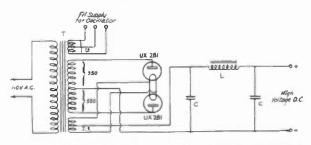
CIRCUIT DIAGRAM OF THE POWER SUPPLY
