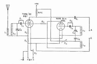
THESE CONNECTIONS ARE USED WITH D.C. TUBES
