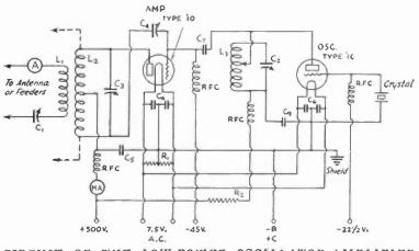
CIRCUIT OF THE LOW-POWER OSCILLATOR-AMPLIFIER SET WITH CRYSTAL CONTROL
