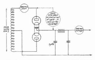
TWO MERCURY-VAPOR TUBES IN A FULL-WAVE CIRCUIT
