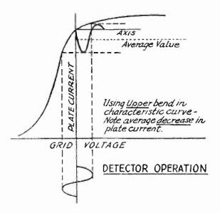
ment current and plate voltage remains constant, the effect on the plate current varies as shown in the diagram. The filament temperature limits in the emission of electrons causing the bend at the top of the curves, as saturation is approached. The bends (A, B, C, D in the curves of amplifier operation) can be used for detection. The straight section of the characteristic curve is useful for non-distorted amplification.
