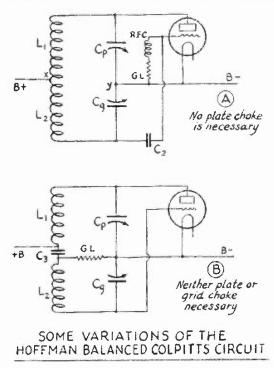
$C_{\rm g}$  should have twice the capacity of  $C_{\rm p}$  to make the grid excitation have the optimum value unless a small grid condenser is used to limit the r.f. grid voltage.
