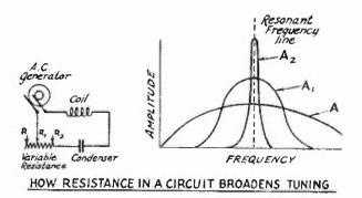
the circuit. We get the loudest signals with a receiver having low resistance circuits and we get the highest efficiency in a transmitter when the resistance of the tuned circuits is at a minimum, other things being equal.
