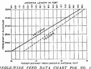
SINGLE-WIRE FEED DATA CHART FOR NO. 14 WIRE FEEDER
