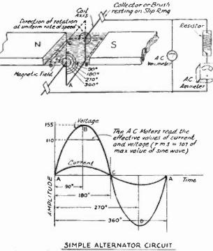
Diagram shows instantaneous values of current and voltage with electrical degrees of coil rotation – there are 360 clectrical degrees for every pair of poles so that one complete mechanical revolution may correspond to more than one clectrical revolution.
