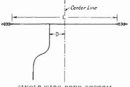
SINGLE-WIRE FEED SYSTEM The length L and coupling D are determined from the chart.
