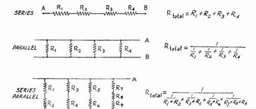
RESISTANCES CONNECTED IN SERIES, PARALLEL, AND SERIES-PARALLEL
