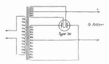
CONNECTIONS USED WITH A TYPE '80 TUBE
