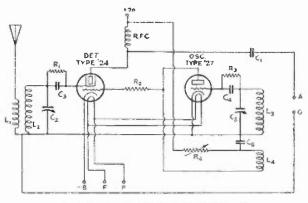
WIRING OF THE CONVERTER
