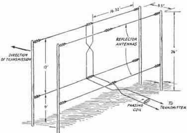
A 28-MC. DIRECTIVE ANTENNA SYSTEM Four in-phase antennas backed up by four reflectors concentrate the radiation in the direction indicated by the arrow.
