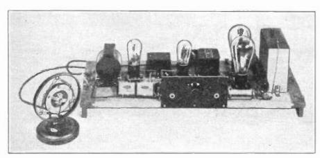
SPEECH AMPLIFIER AND MODULATOR FOR THE LOW-POWER PUSH-PULL CLASS C AMPLIFIER
