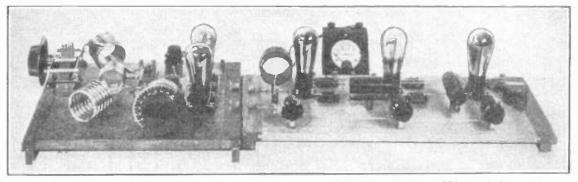
A CRYSTAL-CONTROLLED TRANSMITTER WITH TWO FREQUENCY DOUBLERS The push-pull amplifier is the one previously described. The oscillator is at the extreme right with the frequency doublers to its left. "Midget" type variable condensers are used for tuning the oscillator and doubler tank circuits.
