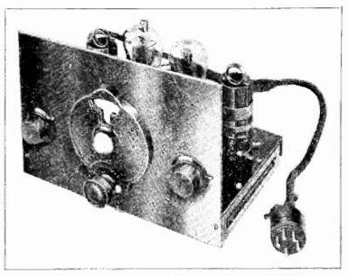
A SUPERHET CONVERTER FOR A.C. OPERATION The small knob at the left is the detector tuning control, the dial in the center the oscillator tuning, and the knob at the right the regeneration control.
