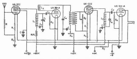
THE CONNECTIONS OF THE FOUR-TUBE RECEIVER
