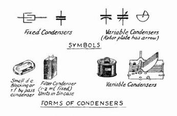
thing being rolled into compact form and enclosed in a metal can. Common units of this type have capacities between one and four microfarads.
