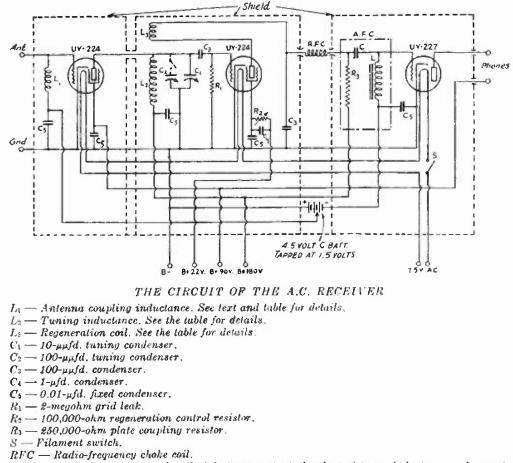
AFC — Audio-frequency coupler. Satisfactory constants for the resistance, inductance and capacitance are, respectively: Rs, 250,000 ohms; L, 30 henries; C, 0.01 µfd.
