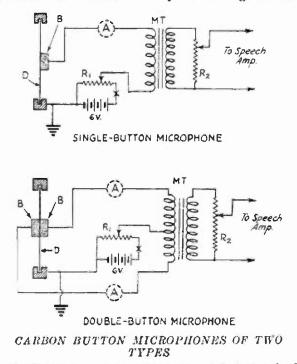
The diaphragms are designated by D and the buttons by B.  $R_1$  may be 400 ohms and the gain control  $R_2$  a 100,000-ohm potentiometer. The microphone frame should be grounded and the leads should be shielded to prevent r.f. pick-up.
