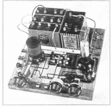
AN EXPERIMENTAL MODEL OF THE MODULOMETER The non-inductive resistor is to the left of the variable condenser. The d.p.d.t. switch in the center is for changing from "audio input" to r.f. input for the measurement of percentage of modulation.
