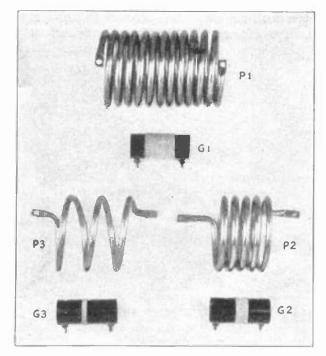
THE PLATE AND GRID COILS
