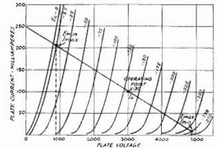
MODULATOR LOAD LINE FOR 100% MODULATION PLOTTED ON THE PLATE CHARACTERISTIC CURVES OF A TYPE '49 TUBE
