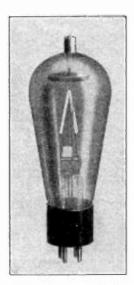
A TYPICAL HOT-CATHODE MERCURY-VAPOR RECTIFIER TUBE
