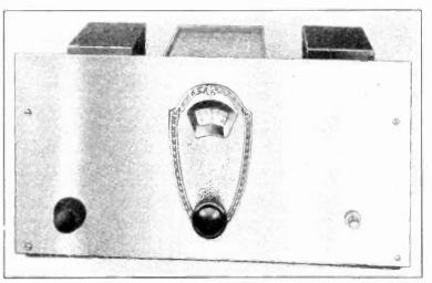
PANEL VIEW OF THE THREE-TUBE A.C. RECEIVER The tuning dial is in the center. The small knob at the left is the regeneration control, and the switch at the right is in the filament circuit.
