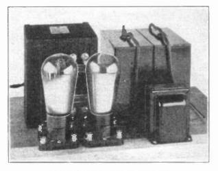
COMPLETE POWER SUPPLY For a transmitter using one or two Type '10 tubes.
