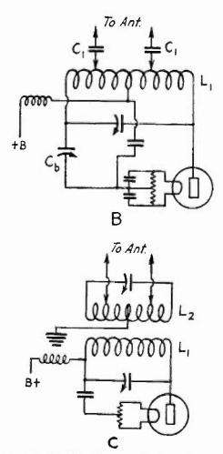
THREE ARRANGEMENTS FOR COUPLING THE TRANSMISSION LINE TO THE TRANSMITTER
