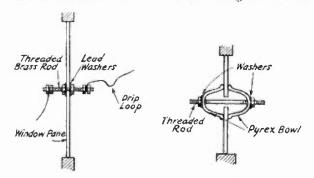
TWO GOOD METHODS OF BRINGING THE TRANS-MITTING ANTENNA LEAD-IN THROUGH A WINDOW
