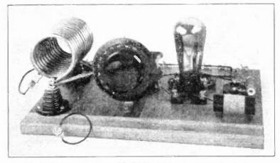
THE SINGLE-CONTROL LOW-POWER TRANSMITTER The plate tank circuit is at the left. The grid coil, leak and grid condenser are to the right of the Type '10 tube.
