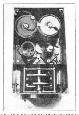
PLAN VIEW OF THE CALIBRATED MONITOR In this instrument particular care was taken to obtain mechanical rigidity and generally substantial construction. The switching arrangement for throwing in any of the three possible capacity values can be seen between the tube and the coil. The shield of this monitor is made of heavy copper plate built up on aluminum anale-pieces.
