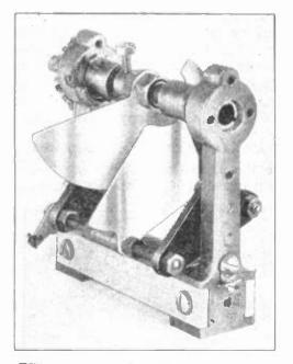
THE "SLIDING ROTOR" CONDENSER The space which each band occupies on the dial can be adjusted by changing the spacing between the rotor and stator plate.
