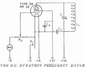
L1 - 75 turns of No. 30 d.c.c. wire on 1/2-inch form, no spacing
