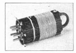
TYPICAL COIL CONSTRUCTION WITH MANU-FACTURED FORMS
