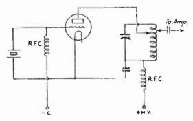
THE POWER CRYSTAL OSCILLATOR CIRCUIT The plate tap on the tank inductance permits control of the grid excitation.
