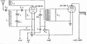
THE SIMPLE WIRING OF THE TWO-TUBE SET Apparatus required:
