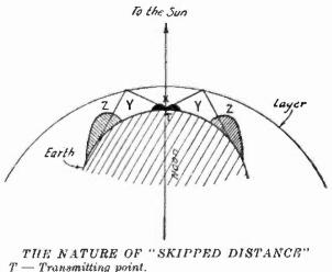
$X \rightarrow$  Local signal due to earth-bound or ground wave.
