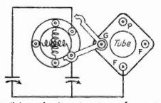
Wiring of coil and setting of switch to connect larger section of condenser across grid coil for the Tooo-K.c. band.
