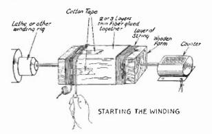
wooden block should be slightly larger than the leg of the core on which the winding is to be put and it should be a few inches longer than the winding. The block must be smooth and of just the right size. Several pieces fastened with small screws at the ends will make a form which can be easily taken apart when the winding is finished.
