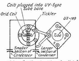
Wiring of coil and setting of switch for the 14,000-K.C. band.
