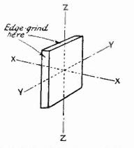
RELATION OF THE AXES OF AN X-CUT QUARTZ PLATE
