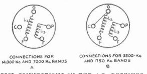
COIL CONNECTIONS IN THE A.C. RECEIVER
