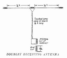
(lamp-cord) as a feeder and loosely coupled to the input inductance of the receiver by a tuned or untuned coupling coil. The dimensions of the antenna and feeder components correspond with those of the transmitting antennas of a similar type which are described later.
