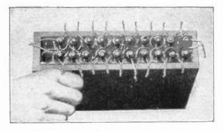
A COMPLETE RECTIFIER FOR 750 VOLTS The organic-solution type of cell is used. The photograph shows how compact the whole assembly may be made.
