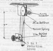
Wind the dial cord around both drums about 4 times and position the light tension spring to the upper right (front view) with the loop condenser fully anti-clockwise.
