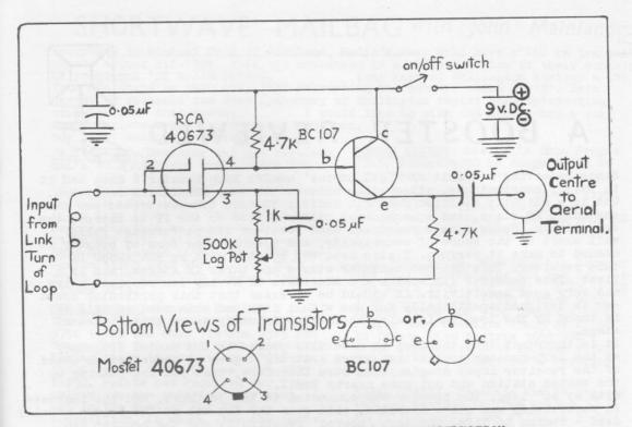
very small and consequently there is very little current drawn from the battery, and it should last for three to four months at least, left running, while the addition of a switch will extend its life further.
