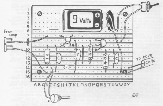
Components are shown on this diagram as though they are mounted on the copper striped side of the Veroboard. This is purely for illustration purposes.
