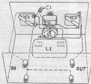
For convenience & clarity, wires between coil L1 and switch S2 are not shown. See separate diagram of these two components. Wires are shown in approx positions only. Solid dot represents a soldered connection.
