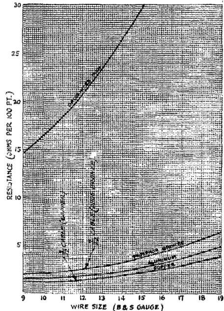
FIG. 2 RADIO FREQUENCY RESISTANCE OF WIRES AT 200 METERS
