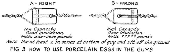
then as in Fig. 3B. The losses when used as at A were about 1/5 as great. Tests were then made with two eggs in series. When they were connected with wire they consumed 1 watt when dry and 5 watts when wet but when connected with rope they consumed 19 watts when dry and 24 watts when wet. All this was with the insulators used as in Fig. 3A. Now they were turned as in Fig. 3B and the losses went to 30 watts when dry and 47 watts when wet.
