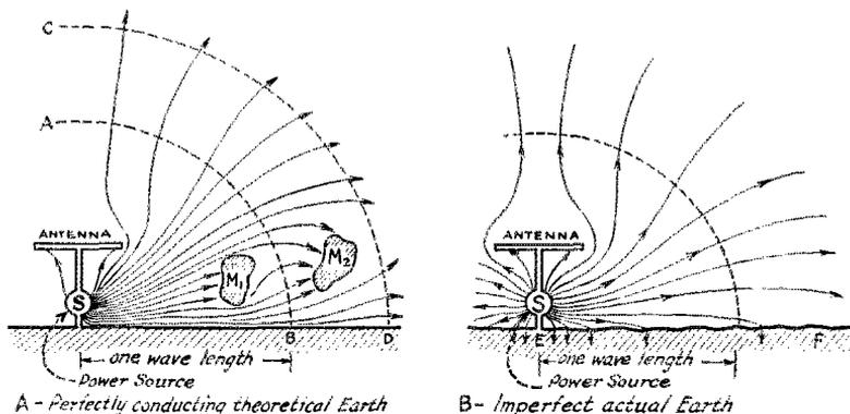
FIG. 1 - FLOW OF POWER FROM AN ANTENNA
