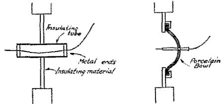
M. B. West in one case found that the removal of a very large composition lead-in insulator decreased the antenna capacity by 10%. At WWV a 20% increase in antenna current was obtained by taking out a very good electrose bushing and running the lead thru the center of a window-pane.
