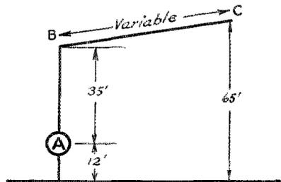
The test antenna at 1XT-1QP
