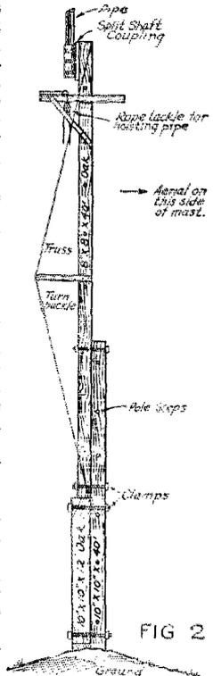
the lower end of the pipe and wired into place. To couple on another section of pipe the clamp at the top of the wooden mast was tightened, the rope slacked off and the pulley lowered to pick up the new section.
