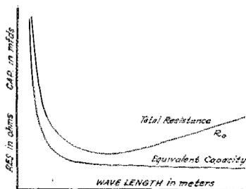
FIG. 1 Curves of Total Resistance and Equivalent Capacity
