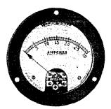
Direct Current Ammeter for Radio Application
