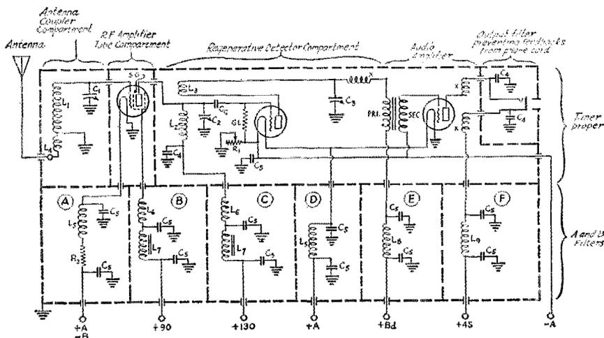
FIGURE 2. THE COMPLETE DIAGRAM OF THE SET
