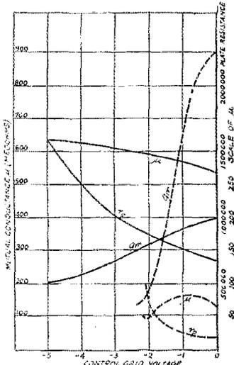
UX 222 EFFECT OF CONTROL GRID BIAS ON  $G_m$ ,  $\mu$  AND  $\mu_p$  FOR BOTH SHIELD-GRID AND SPACE-CHARGE METHODS OF OPERATION, THE CONTROL GRID IN EACH CASE BEING THE ONE APPROPRIATE FOR THE METHOD.
