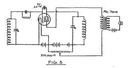
a space charge detector. A stage of transformer coupled audio amplification followed. Signal strength was not much, if any, better than that obtained with a 201-A in the same circuit. Resistance coupling to the audio tube was also tried with no better results, a Clarostat being used as a combined coupling resistance and plate voltage control.
