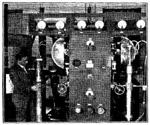
THE 50-KW. LINEAR AMPLIFIER WITH THE FRONT-DOORS OPEN
