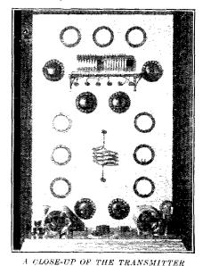
The jour crustals are mounted in the square backs on the bottom shelf. The oscillator is the tube at the left; the tube at the right is the first frequency doubler. The tank and satema inductances are conveniently mounted and ready for changing. The use of the various meters is described in the left.
