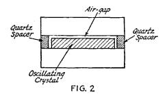
extending over a considerable period, the frequency of the transmitter did not vary in excess of 20 cycles from the assigned frequency. The 20cycle shift occurred during the first hour, after which zero beat was maintained for the remaining hours of the test. The temperature of the oven varied over a range of approximately  $1.8^{\circ}$  (C.) during the run.
