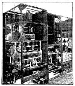
A PEEK AT THE REAR OF THE 5-KW. STAGE The plate inductance and the yrid coupling coil for the 50-kw, stage input are on the second deck from the bottom. The toasterlike appearing rig on the third deck is the Ohm-spun prid-shund resistor. One of the neutralizing condensers may be seen just in front of the vlate inductance. Part of the rubber tubing coil for cooling water is visible below the first deck.
