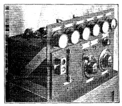
THE CRYSTAL-OSCILLATOR-AMPLIFIER WITH ITS OUTER SHIELD REMOVED
