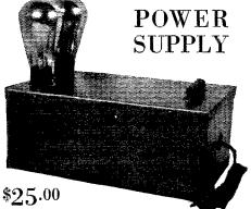
Complete self-contained unit of heavy duty construction using two 281 tubes. Mounted in heavy metal case size 5 x 7 x 12 inches, Wt., 22 lbs. Delivers up to 150 mils at 500 volts filtered D.C. plate supply, also extra 73% V. center tapped filament winding for supplying up to four 210 tubes.
