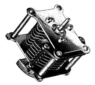
Continued tests under actual operating conditions have shown that the TYPE 334 Variable Air Condensers, formerly rated at 2000 volts, may safely be used on voltages up to 2500, root mean square, or 3500, peak.
