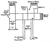
FIG. S. — RELAY AND REMOTE CONTROL CONNECTIONS
